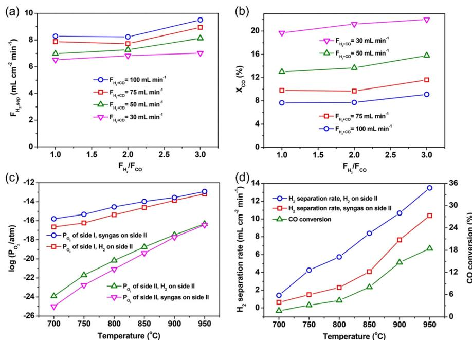
Fig. 12 Effect of the molar ratio of H<sub>2</sub>/CO on the H<sub>2</sub> production rate (a) and CO conversion (b) at different flow rates at 900 °C with BCF-based MOEC membrane reactor. Relationship between temperature and corresponding oxygen partial pressure for both sides of the membrane reactor (c) and H<sub>2</sub> production rate and CO conversion (d). Reproduced with permission from ref. 86. Copyright © 2016, American Institute of Chemical Engineers.
