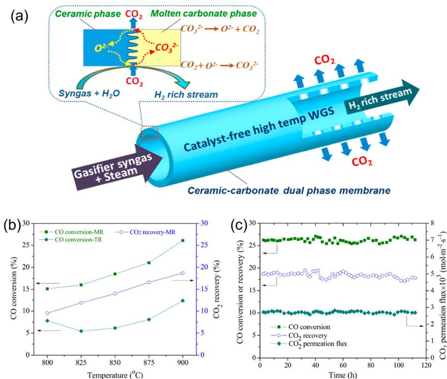
**Fig. 23** MOCC membrane reactor for coupling WGS reaction and CO<sub>2</sub> capture. (a) Schematic diagram, (b) performance of membrane reactor and fixed bed reactor as a function of temperature, and (c) long-term stability of membrane reactor at 900  $^{\circ}\text{C}$ . Reproduced with permission from ref. 123. Copyright © 2016, Elsevier B.V. All rights reserved.
