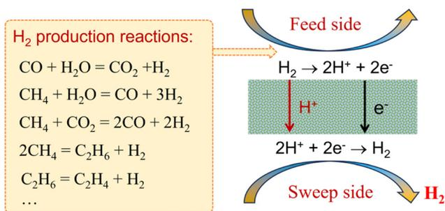
Fig. 2 Schematic of MPEC membrane reactors for coupling H<sub>2</sub> production reactions with H<sub>2</sub> separation.
