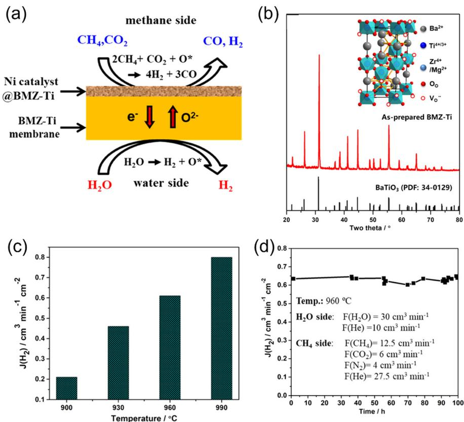
Fig. 16 Hydrogen production from WSR with partial oxidation of methane (POM) reaction on the sweep side with MOEC membrane reactor. (a) Schematic illustration, (b) XRD of BMZ-Ti membrane, (c)  $\text{H}_2$  production rate as a function of temperature and (d) stability test of the BZM-Ti membrane reactor at 960 °C. Reproduced with permission from ref. 89. Copyright © 2021, the American Chemical Society.
