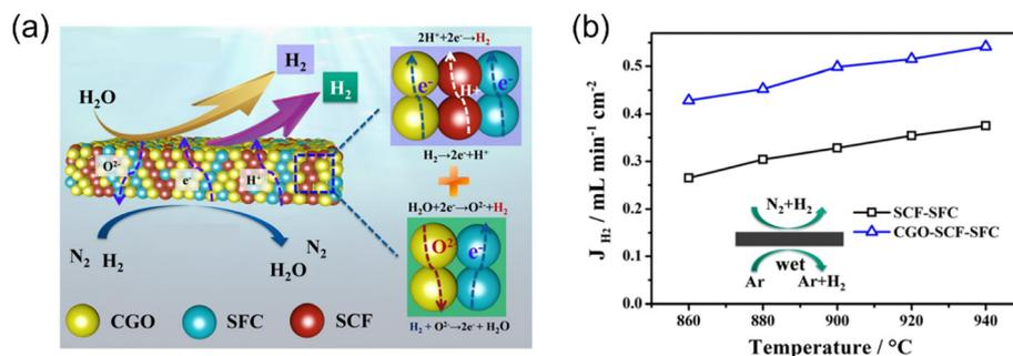
Fig. 11 Hydrogen production from the WSR with low concentration hydrogen as sweep gas in the triple-conducting membrane reactor. (a) Schematic and (b) H<sub>2</sub> production rate of SCF-SFC and CGO-SCF-SFC membrane reactors as a function of temperature. Reproduced with permission from ref. 82. Copyright © 2020, Elsevier B.V. All rights reserved.
