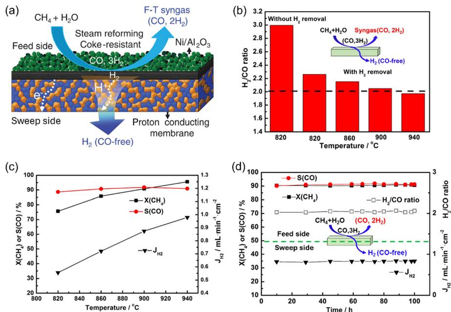
Fig. 4 Hydrogen production from the steam methane reforming (SMR) reaction in the MPEC membrane reactor. (a) Schematic; (b) H<sub>2</sub>/CO ratio and (c) CH<sub>4</sub> conversion, CO selectivity and H<sub>2</sub> production rate as a function of temperature; and (d) time dependence of CH<sub>4</sub> conversion, CO selectivity, H<sub>2</sub> production rate and H<sub>2</sub>/CO ratio at 900 °C. Reproduced with permission from ref. 36. Copyright © 2019, American Institute of Chemical Engineers.
