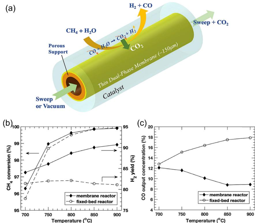
Fig. 25 MOCC membrane reactor for coupling the SRM reaction and CO<sub>2</sub> capture. (a) Schematic, (b) CH<sub>4</sub> conversion and H<sub>2</sub> yield by the membrane reactor and fixed bed reactor as a function of temperature, and (c) CO concentration (dry-based) comparison of the membrane reactor and fixed bed reactor. Reproduced with permission from ref. 124. Copyright © 2019, Elsevier B.V. All rights reserved.
