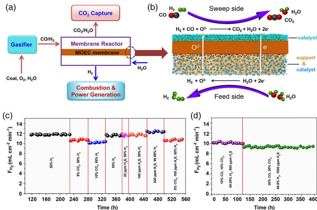
Fig. 14 Schematic of the IGCC-MOEC process and stability test. (a) Illustration of the IGCC-MOEC process. (b) Coupling  $\text{H}_2$  production, syngas oxidation, and  $\text{CO}_2$  capture in an MOEC membrane reactor. (c and d)  $\text{H}_2$  production rates during the long-term stability tests under various atmospheres at  $900^\circ\text{C}$ . Reproduced with permission from ref. 73. Copyright @ 2020, American Institute of Chemical Engineers.
