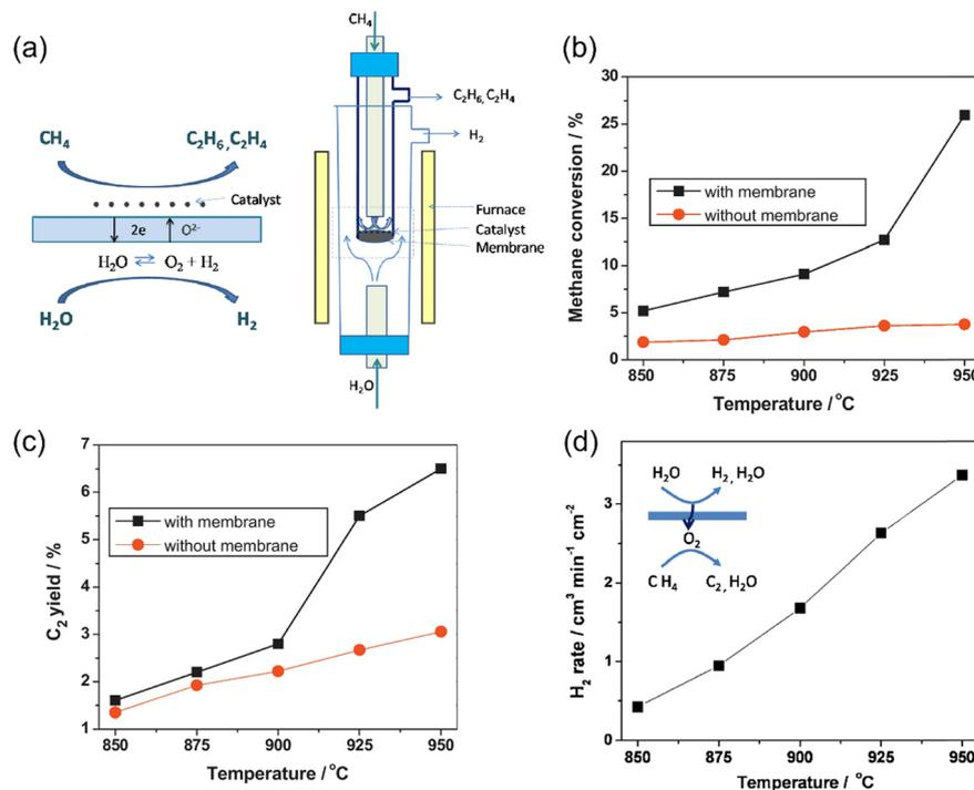
**Fig. 19** Hydrogen production from oxidative methane coupling and water splitting in MOEC membrane reactor. (a) Schematic illustration, (b) CH<sub>4</sub> conversion with and without membrane as a function of temperature, (c) C<sub>2</sub> yield with and without membrane as a function of temperature, and (d) hydrogen production rate on the feed side as a function of temperature. Reproduced with permission from ref. 81. Copyright © 2011, Elsevier B.V. All rights reserved.
