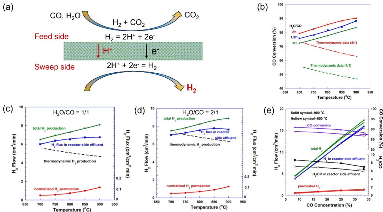
Fig. 3 Hydrogen production from the water gas shift (WGS) reaction in the MPEC membrane reactor. (a) Schematic, (b) CO conversion as a function of temperature, (c and d) H<sub>2</sub> production as a function of temperature with H<sub>2</sub>O/CO = 1/1 and 2/1, and (e) WGS reaction performance in the membrane reactor as a function of CO concentration with H<sub>2</sub>O/CO = 2/1. Reproduced with permission from ref. 38. Copyright © 2012, Elsevier. All rights reserved.
