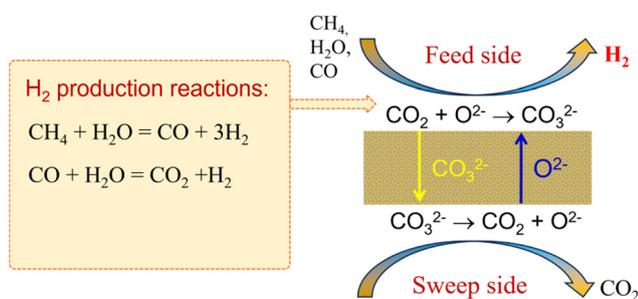
**Fig. 22** Working principle of MOCC membrane reactor for coupling hydrogen production and CO<sub>2</sub> capture.
