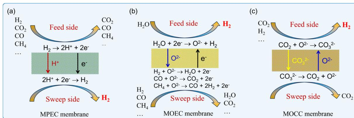
Fig. 1 Working principles of three types of ceramic-based membrane reactors for H<sub>2</sub> production: (a) MPEC membrane, (b) MOEC membrane and (c) MOCC membrane.
