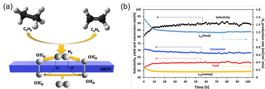
Fig. 7 Hydrogen production from non-oxidative dehydrogenation of ethane in an MPEC membrane reactor. (a) Schematic and (b) stability test at 700 °C. Reproduced with permission from ref. 26. Copyright © 2020, Elsevier B.V. All rights reserved.
