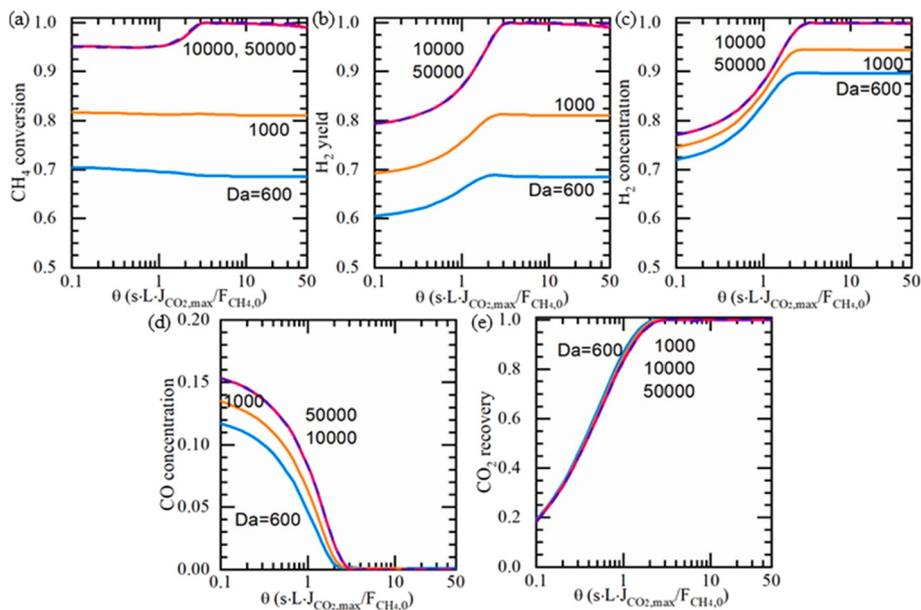
**Fig. 26** Simulation results of (a) CH<sub>4</sub> conversion, (b) H<sub>2</sub> yield, (c) H<sub>2</sub> concentration, (d) CO concentration, and (e) CO<sub>2</sub> recovery, when 5 atm and 10<sup>-3</sup> vacuum sweep are applied. At 800 °C, S/C = 3, sweep/feed flow rate ratio = 100. Dry-based molar concentration calculation. Reproduced with permission from ref. 133. Copyright © 2021, Elsevier B.V. All rights reserved.
