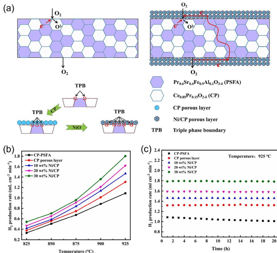
Fig. 15 (a) Schematic diagram of MOEC membrane for oxygen permeation with/without surface modification. (b) Temperature dependence of the  $\text{H}_2$  production rate of the MOEC membrane reactor. (c) Stability test of the MOEC membrane reactor at  $925^\circ\text{C}$ . Reproduced with permission from ref. 79. Copyright © 2022, Elsevier Ltd and Techna Group S.r.l. All rights reserved.
