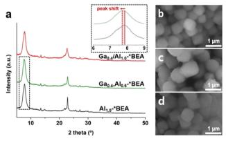
Fig. 1 (a) Powder XRD patterns of  $Ga_{0.4}/Al_{1.0}$ \*BEA,  $Ga_{0.4}$ ,  $Al_{0.6}$ \*BEA, and Al<sub>1.0</sub>-\*BEA (see also Fig. S1 of the ESI† for other samples). Inset: example of the peak shift to lower  $2\theta$  with isomorphic Ga substitution. (b-d) Scanning electron microscope (SEM) images of representative (b)  $Ga_{0.4}/Al_{1.0}$ -\*BEA, (c)  $Ga_{0.4}$ ,  $Al_{0.6}$ -\*BEA, and (d)  $Al_{1.0}$ -\*BEA samples.
