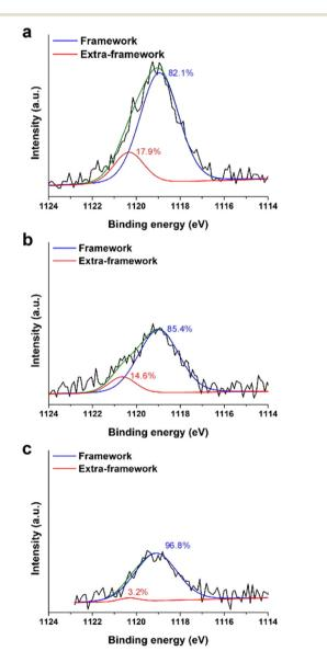
Fig. 2 XPS spectra of Ga  $2p_{3/2}$  for (a)  $Ga_{0.6}$ ,  $Al_{0.6}$ -\*BEA, (b)  $Ga_{0.4}$ ,  $Al_{0.6}$ -\*BEA, and (c) Ga<sub>0.2</sub>,Al<sub>0.6</sub>-\*BEA samples. Peak positions are corrected using a carbon reference. Peak deconvolution was executed using Gaussian fits to obtain relative percentages (listed) of framework (blue) and extra-framework (red) Ga species (see also Table S5 of the ESI†). Green lines refer to fitted composite spectra.
