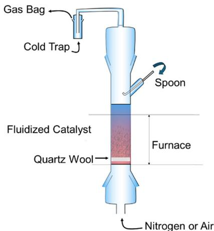
Fig. 1 FCC reactor for the ChemPren process.
