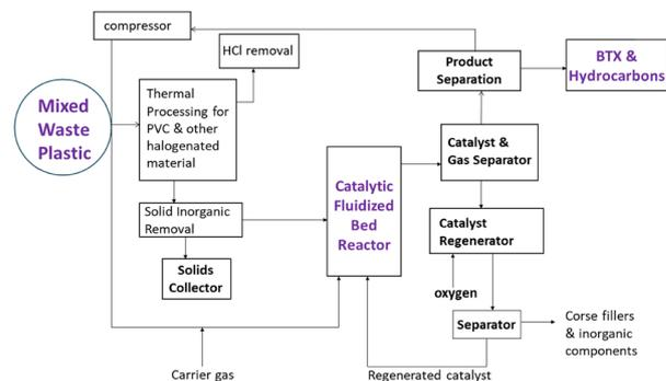
Fig. 2 Block flow diagram of the ChemPren process.
