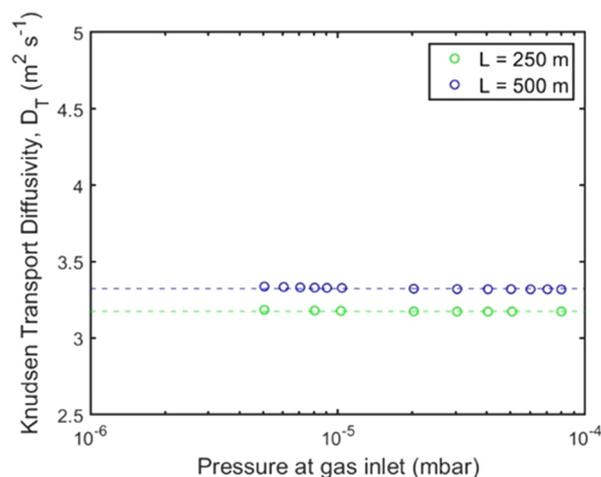
**Fig. 5** Knudsen transport diffusivity for the channels with 250 mm (green) and 500 mm (blue) length for varying pressure gradient at the gas inlet using the UHVDS.
