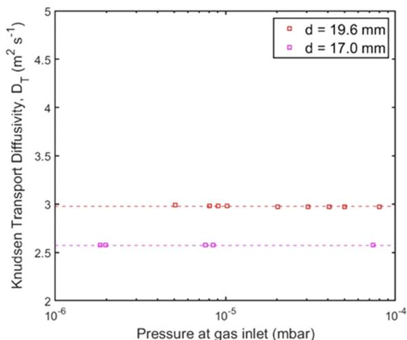
**Fig. 10** Knudsen transport diffusivity for the square channels with 19.6 mm (red squares) and 17.0 mm (pink squares) hydraulic diameter and 500 mm length for varying pressure at the gas inlet using the UHVDS.
