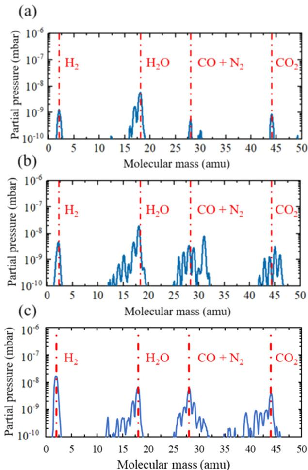
**Fig. 8** Mass spectral analysis of the gas species that are present in the UHVS: (a) “empty” system; (b) a pre-treated PA2200 nylon segment of  $L = 50$  mm fabricated by the SLS EOS Formiga P100 3D printer, and (c) a pre-treated high-temperature resin channel of  $L = 500$  mm fabricated by the SLA Formlabs Form 3 3D printer inserted inside the diffusion channel. The analysis is conducted using the SRS RGA100 mass spectrometer.
