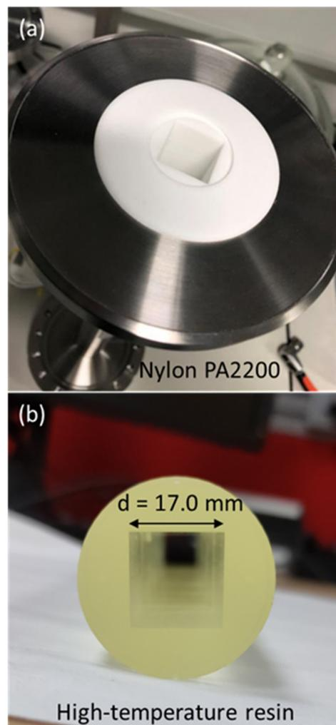
**Fig. 9** Photographs of two channels with a square cross section with edge length of 17 mm and channel length of 500 mm, made of: (a) PA2200 nylon using an SLS EOS Formiga P100 3D printer, and (b) high-temperature resin using an SLA Formlabs Form 3 3D printer.
