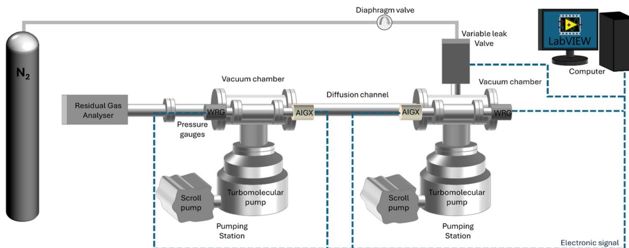
Fig. 1 Schematic representation of the UHVDS and its components.
