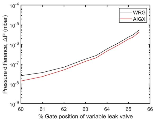
**Fig. 3** Pressure difference generated between the two sides of the diffusion channel as measured by the WRG (black) and AIGX (red) pressure gauges depending on the gate position of the leak valve. The gate position of the valve can be linked with the applied molar flux.
