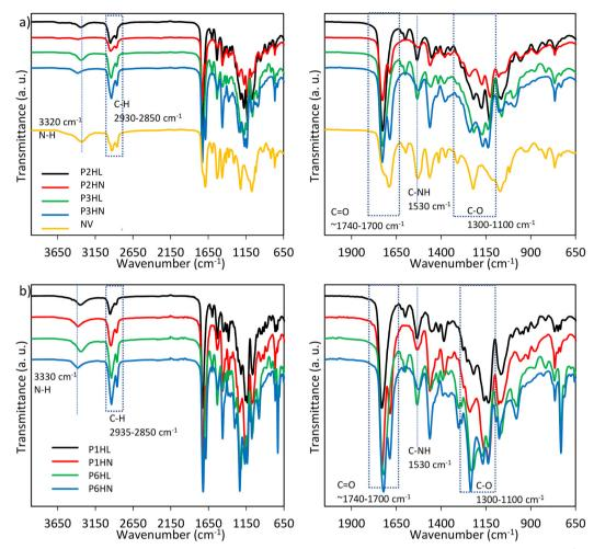
Fig. 3 FT-IR spectra of PUR adhesives: a) P2HL, P2HN, P3HL, P3HN, NV; b) P1HL, P1HN, P6HL, P6HN; zoom region (1950–650 cm<sup>-1</sup>) on the right side.
