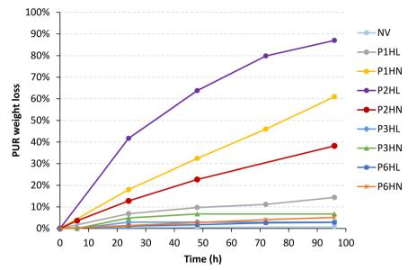
Fig. 4 Weight loss (%) by cutinase HiC (100 U mL<sup>-1</sup>) of PUR adhesives, as a function of the incubation time (hours).
