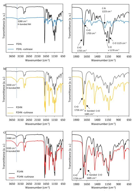
Fig. 5 FT-IR spectra of degraded PUR adhesives: a) P2HL, b) P2HN, c) P1HN; zoom region (1950-650 cm<sup>-1</sup>) on the right side.
