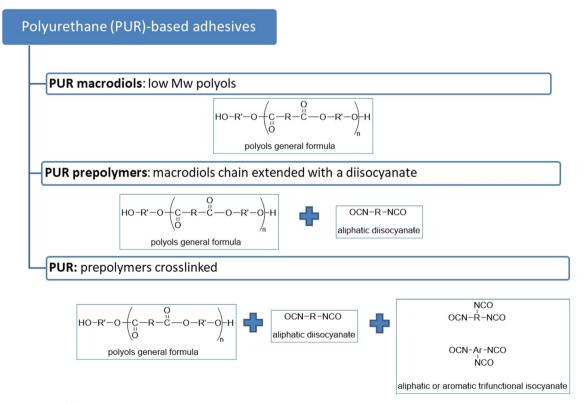
Fig. 1 General scheme of PUR
