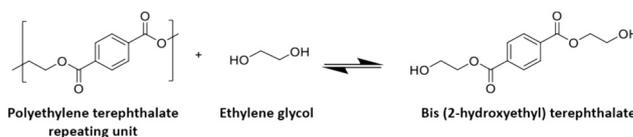
Fig. 1 Depolymerization reaction of PET with EG into BHET.
