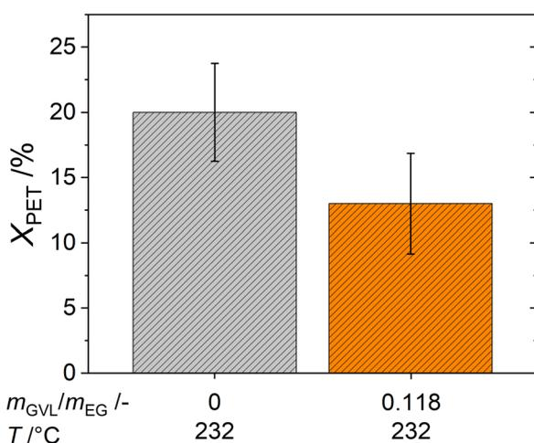
**Fig. 6** PET conversion  $X_{PET}$  of samples without catalyst after 7 minutes of reaction time without GVL (light grey shaded) and with  $\frac{m_{GVL}}{m_{EG}} = 0.118$  (orange shaded) at  $T = 232$  °C,  $p = 3$  bar,  $\frac{m_{EG}^0 + m_{GVL}}{m_{PET}^0} = 6$ ,  $0.2 \leq d_p < 1$  mm and a stirrer speed of 1400 rpm.
