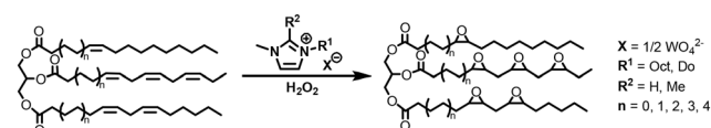
Scheme 2 Catalytic two-phase epoxidation of vegetable oils with imidazolium tungstate SAILs as catalysts and aq. H 2 O 2 as the oxidant.
