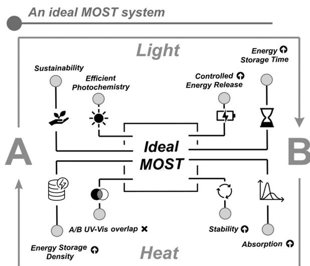
Fig. 2 Key features of an ideal MOST system.
