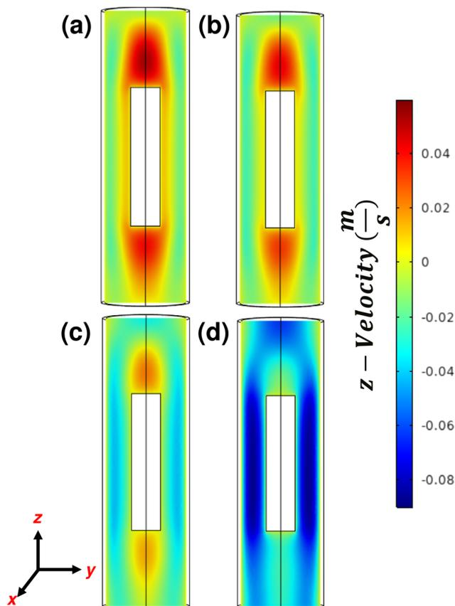
Fig. 4 Axial velocity on the ZY plane of the heating element with 30 V applied and He inlet flow rate of (a) 90 mL min<sup>-1</sup>, (b) 180 mL min<sup>-1</sup>, (c) 360 mL min<sup>-1</sup>, and (d) 720 mL min<sup>-1</sup>.
