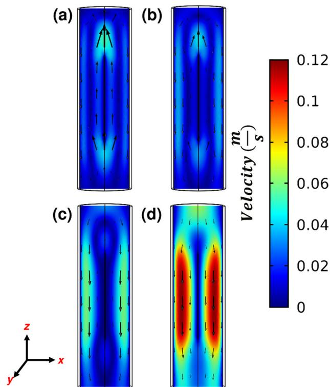
Fig. 5 Velocity magnitude and direction of flow on the plane perpendicular (XZ plane) to the heating element with 30 V applied and He inlet flow rate of (a) 90 mL min<sup>-1</sup>, (b) 180 mL min<sup>-1</sup>, (c) 360 mL min<sup>-1</sup>, and (d) 720 mL min<sup>-1</sup>.
