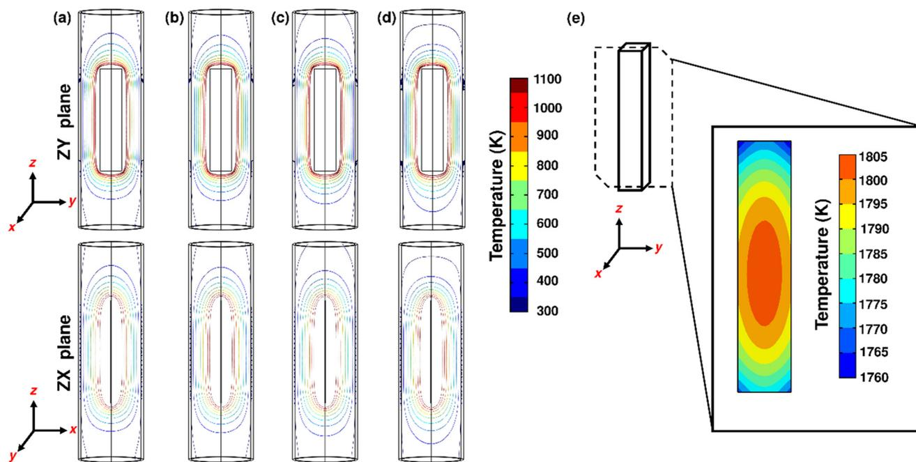
Fig. 2 Temperature isotherms at steady state for 30 V applied for a He inlet flow rate of (a)  $90 \text{ mL min}^{-1}$ , (b)  $180 \text{ mL min}^{-1}$ , (c)  $360 \text{ mL min}^{-1}$ , and (d)  $720 \text{ mL min}^{-1}$ . (e) Temperature contours of the element surface (ZY plane) at steady state for 30 V applied.
