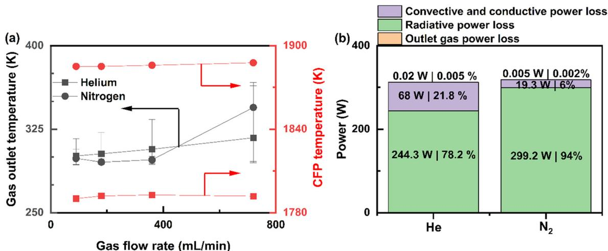
Fig. 3 Steady state temperature and power distribution. (a) Average element and average gas outlet temperatures at steady state vs. gas flow rate. Conditions: 30 V (error bars represent the maximum and minimum gas outlet temperature). (b) Power distribution when a power of ~312 W is applied to CFP, at steady state, using N<sub>2</sub> or He, each with an inlet flow rate of 90 mL min<sup>-1</sup>.
