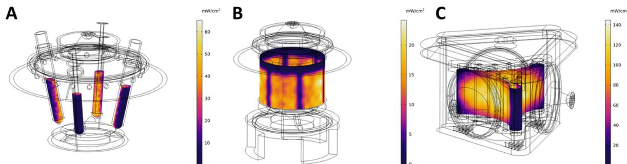
**Fig. 4** Simulated irradiation profiles mapped on the irradiated surfaces for the 4-vial UFO reactor (A), the Uflow reactor (B) and the Fidget reactor (C). These profiles were generated for one Kessil PR160L-370 nm at 100% intensity setting, three lamps in the Fidget reactor simulation. The wireframe visualization shows the general geometry of the reactors as per design.
