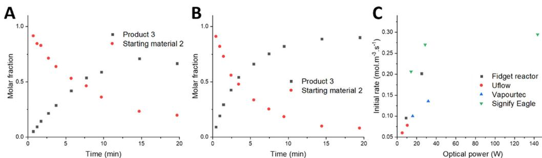
**Fig. 6** A) Evolution of the reaction composition (molar fraction based on reagent 2 and product 3) at different reaction times in the Uflow reactor. B) Evolution of the reaction composition (molar fraction based on reagent 2 and product 3) at different reaction times in the Fidget reactor. C) Initial rate of the chemical transformation at different optical power for the different reactor designs.
