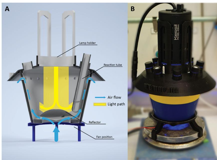
**Fig. 1** A) Sliced schematic design of the UFO batch reactor system with air flow and light path directions indicated. B) Assembled 8-vial UFO reactor being operated, mounted on a custom clamp support to fit IKA magnetic stirring plates.
