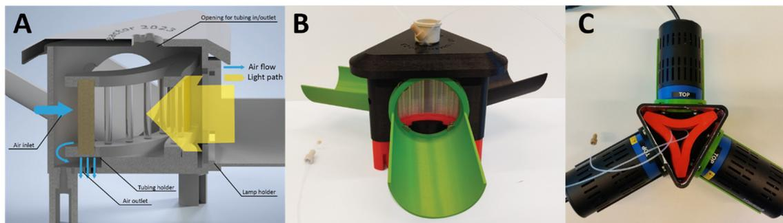
**Fig. 3** A) Sliced schematic design of the Fidget reactor system with air flow and light path directions indicated. B) Assembled reactor system built and ready for operation, showing the wound capillary in its custom holder. C) Top view of the opened Fidget reactor equipped with the 3 Kessil lamps.
