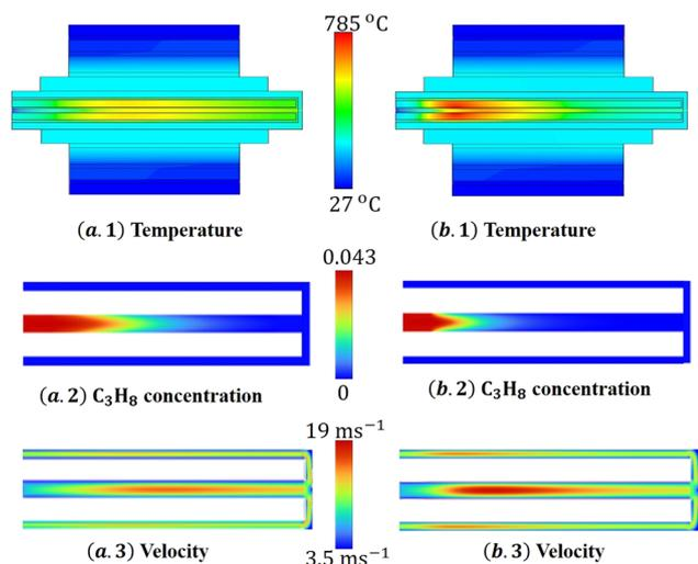
**Fig. 6** The effect of the inner wall material on the contours of temperature (top), propane mass fraction (middle) and velocity (bottom). The inner dividing of the S-HRR wall is steel in the left panels (a.1–a.3) and ceramic in the right panels (b.1–b.3). In the middle and bottom panels, only the flow channels of S-HRR are shown. The inlet velocity is  $3.5 \text{ ms}^{-1}$ ,  $\phi = 0.7$  and other conditions the same as in Fig. 2.
