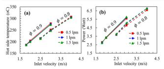
Fig. 3 Plot shows the temperatures on the hot-side of TEG module (a) at various inlet velocities and equivalence ratios of 0.8 (dashed lines) and 0.9 (solid lines) at three different cooling water flow rates of 0.5,1 and 1.5 lpm indicated by squares, circles, and triangles respectively. (b) shows the power generated from the TEGs coupled on either side of S-HRR at corresponding operating points.
