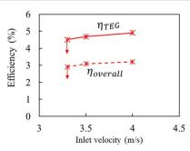
Fig. 5 Thermoelectric ( $\eta_{TEG}$ , solid line) and overall ( $\eta_{overall}$ , dashed line) efficiencies of the S-HRR-TEG coupled with a water-cooled heat sink, at  $\phi = 0.7$  and various inlet velocities.
