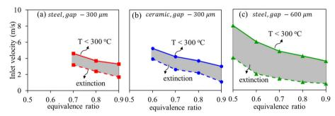
Fig. 12 Comparison of the operating regimes of the integrated device for (a) steel/300 μm; (b) ceramic/300 μm; and (c) steel/600 μm, where steel or ceramic represent material of the inner wall and the number represents the gap-size of the outer recirculation channels. The lower branch (dashed lines) indicates the extinction limit and the upper branch (solid lines) indicates the velocities that limit the skin temperatures below 300 °C.
