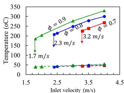
**Fig. 2** Temperatures at the hot-side (solid lines) and cold-side (dashed lines) on the TEG module at equivalence ratios of 0.7 (squares), 0.8 (circles), and 0.9 (triangles) and a cooling water flow rate of 0.51 lpm (equivalent to an inlet velocity of 0.27 ms<sup>-1</sup>). Downward arrows indicate extinction velocities at corresponding equivalence ratios.
