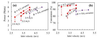
Fig. 8 (a) Power generated and (b) and propane conversion from the coupled device, when the inner walls of the S-HRR are made of steel (solid line) and ceramic (dashed line). Two different equivalence ratios,  $\phi$  = 0.7 (squares) and  $\phi$  = 0.6 (diamonds) are considered. Downward arrows indicate extinction velocities.
