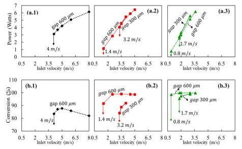
Fig. 11 (a.1-a.3) The net power generated and (b.1-b.3) propane conversion from the integrated device for the gap-widths of recirculation channel of 300  $\mu$ m (solid line) and 600  $\mu$ m (dotted line) at equivalence ratios of  $\phi = 0.5$  (left), 0.7 (mid), 0.9 (right).
