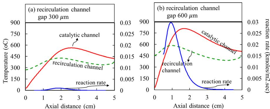
**Fig. 10** Temperature profiles along the centerlines of the catalytic (solid lines) and the recirculation (dashed lines) channels of the S-HRR when the gap-size of the recirculation channel is (a) 300  $\mu\text{m}$  and (b) 600  $\mu\text{m}$ . The other conditions are the same as Fig. 7.
