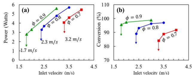
**Fig. 4** (a) Net power generated from the two TEG modules integrated on either side of S-HRR and (b) propane conversion vs. inlet velocity. The three curves represent different values of equivalence ratios. The operating conditions are the same as those in Fig. 2.
