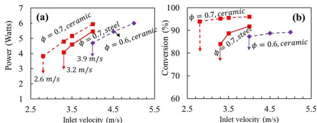
**Fig. 8** (a) Power generated and (b) propane conversion from the coupled device, when the inner walls of the S-HRR are made of steel (solid line) and ceramic (dashed line). Two different equivalence ratios,  $\phi = 0.7$  (squares) and  $\phi = 0.6$  (diamonds) are considered. Downward arrows indicate extinction velocities.
