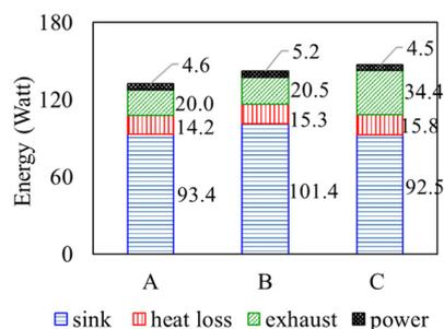
**Fig. 13** Analysis of energy associated with various streams: (A) steel/300  $\mu\text{m}$ , (B) ceramic/300  $\mu\text{m}$ , and (C) steel/600  $\mu\text{m}$  at the inlet velocity 3.5  $\text{ms}^{-1}$  and equivalence ratio of 0.7. As before, steel or ceramic are materials of the inner channels, and the number represents gas-width of the recirculation channel.
