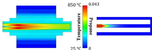
**Fig. 9** Effect of increased gap-size of the recirculating channel to 600  $\mu\text{m}$  on contours of temperature and propane mass fraction. All other conditions are as in Fig. 6(a), with only the recirculation channel width increased from 300 to 600  $\mu\text{m}$ .
