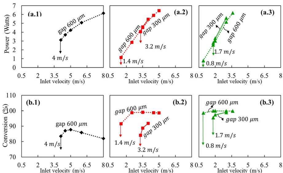
**Fig. 11** (a.1–a.3) The net power generated and (b.1–b.3) propane conversion from the integrated device for the gap-widths of recirculation channel of  $300 \mu\text{m}$  (solid line) and  $600 \mu\text{m}$  (dotted line) at equivalence ratios of  $\phi = 0.5$  (left),  $0.7$  (mid),  $0.9$  (right).
