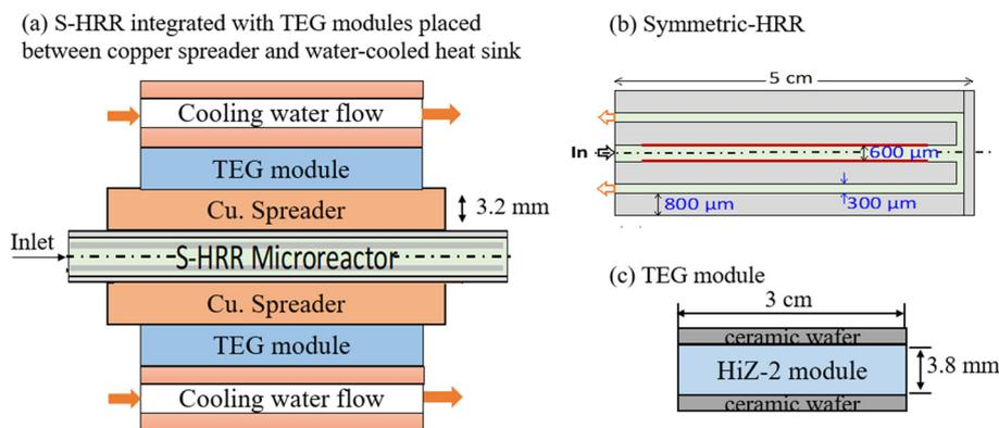
**Fig. 1** Schematic of an integrated device comprising S-HRR integrated with TEG modules on either side, placed between the copper spreader and water-cooled copper heat sink (a). The reactants enter the reactor through the central inlet channel, which is catalyst coated (indicated by thick red lines), and exit through the recirculation channels on either side as directed by the arrows (b). Hi-Z TEG module with semiconductor assembly sandwiched by ceramic wafers on either side is shown in (c).
