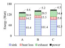
Fig. 13 Analysis of energy associated with various streams: (A) steel/  $300~\mu m$ , (B) ceramic/ $300~\mu m$ , and (C) steel/ $600~\mu m$  at the inlet velocity  $3.5~ms^{-1}$  and equivalence ratio of 0.7. As before, steel or ceramic are materials of the inner channels, and the number represents gas-width of the recirculation channel.
