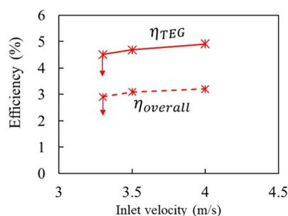
**Fig. 5** Thermoelectric ( $\eta_{\text{TEG}}$ , solid line) and overall ( $\eta_{\text{overall}}$ , dashed line) efficiencies of the S-HRR-TEG coupled with a water-cooled heat sink, at  $\phi = 0.7$  and various inlet velocities.
