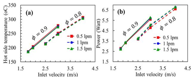
**Fig. 3** Plot shows the temperatures on the hot-side of TEG module (a) at various inlet velocities and equivalence ratios of 0.8 (dashed lines) and 0.9 (solid lines) at three different cooling water flow rates of 0.5, 1 and 1.5 lpm indicated by squares, circles, and triangles respectively. (b) shows the power generated from the TEGs coupled on either side of S-HRR at corresponding operating points.
