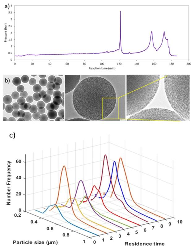
**Fig. 9** a) Pressure profile of reaction system, b) HR-TEM images of MSPs (average size  $490 \pm 9 \text{ nm}$ ), and c) particle size distribution obtained at each residence time cycle (mean residence time is 20 min and the numbers on the axis indicate multiples of mean residence time) using slug flow at  $T_G = 55 \text{ }^\circ\text{C}$ , 25%  $\text{N}_2$  flow rate, and  $0.0045 \text{ M}$  NaOH.
