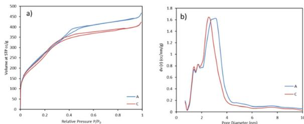
**Fig. 4** a) BET adsorption and desorption isotherms and b) pore size distribution calculated by the DFT method (A = reaction performed without pulse,  $T_G = 55\text{ }^\circ\text{C}$ , C = pulse of methanol given for 5 s@88 ml  $\text{min}^{-1}$ ,  $T_G = 45\text{ }^\circ\text{C}$ ).
