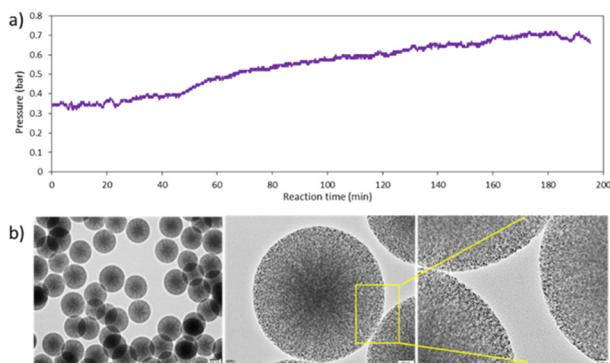
**Fig. 7** a) Pressure profile of the reaction system using slug flow 25%, and b) HR-TEM images of MSPs obtained using slug flow at  $35 \text{ }^\circ\text{C}$ , 25%  $\text{N}_2$  flow rate, NaOH  $0.0045 \text{ M}$ .
