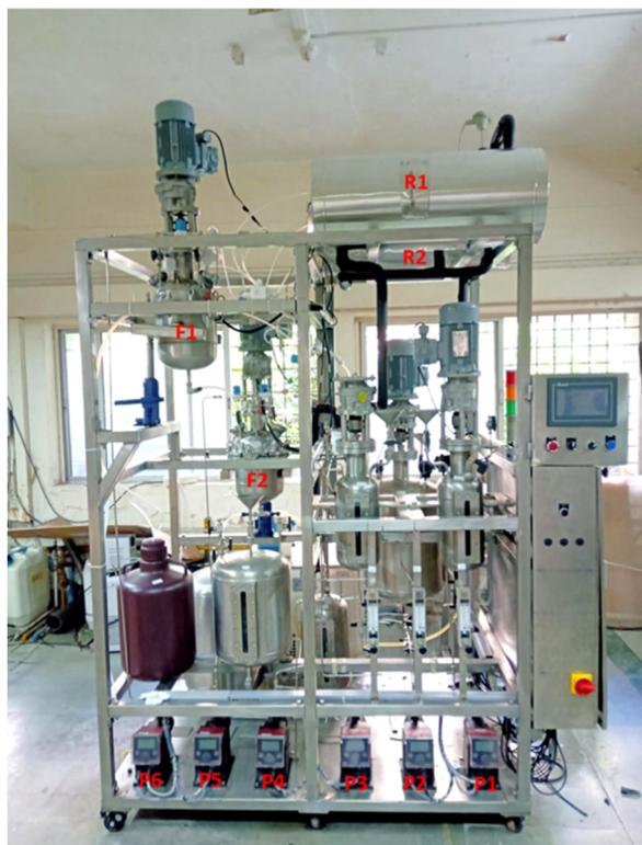
**Fig. 1** Photograph of the mesoporous silica pilot plant for continuous production at a capacity of 1 kg per day. (P1 to P6) pumps, (R1, R2) helical coiled tubular reactor, and (F1, F2) two stage continuous filtration unit.
