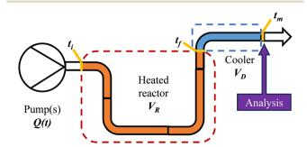
Fig. 2 Diagrammatic representation of a generic flow reactor system with a dead volume between reactor and analysis device.
