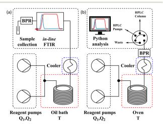
Fig. 5 (a) Schematic of configuration 1 of the flow system utilising an oil bath and in-line FTIR; and (b) schematic of configuration 2 of the flow system utilising an oven and on-line HPLC.
