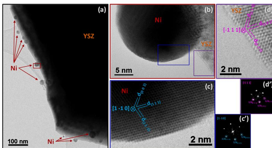
**Fig. 6** TEM images of particles on commercial Ni-YSZ: (a) region with several large Ni particles supported on YSZ. (b) Detailed view of one of those particles. (c) High-resolution image of the surface of the Ni particle in (b) and corresponding 2D-FFT (c'). (d) High-resolution image of the YSZ support surface in (b) and corresponding 2D-FFT (d').
