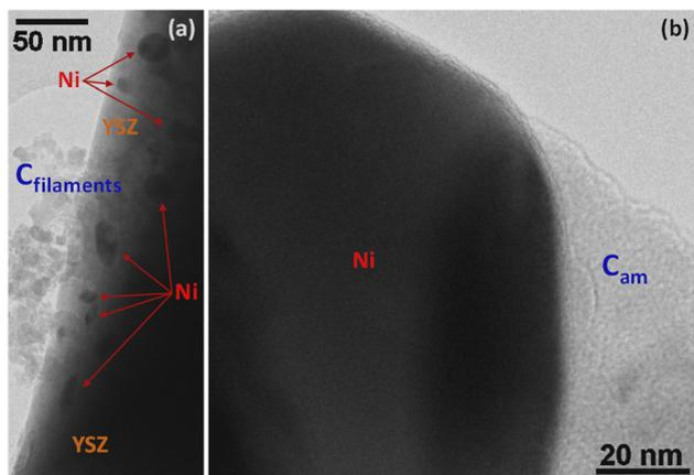
**Fig. 8** TEM images of carbon deposits on commercial Ni-YSZ: (a) region revealing the presence of filamentous carbon ( $C_{\text{filaments}}$ ) near a group of Ni particles supported on YSZ; (b) a thick amorphous carbon ( $C_{\text{am}}$ ) layer partially covers a large Ni particle.
