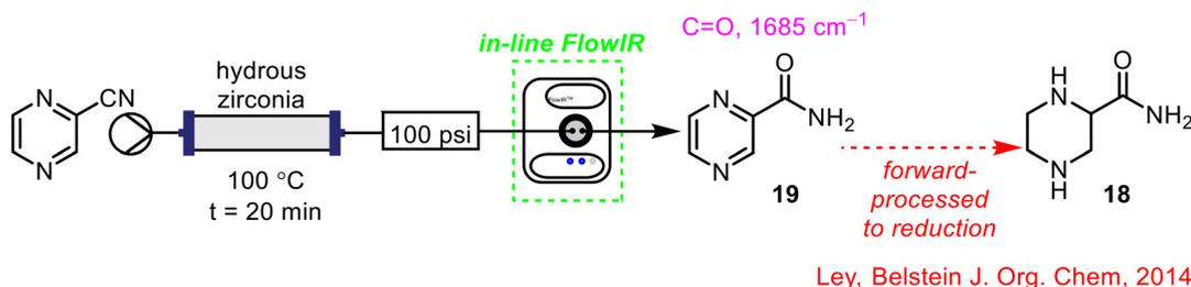
**Scheme 6** Telescoped synthesis of pyrazine-2-carboxamide **18** from **19** using FlowIR.<sup>45</sup>
