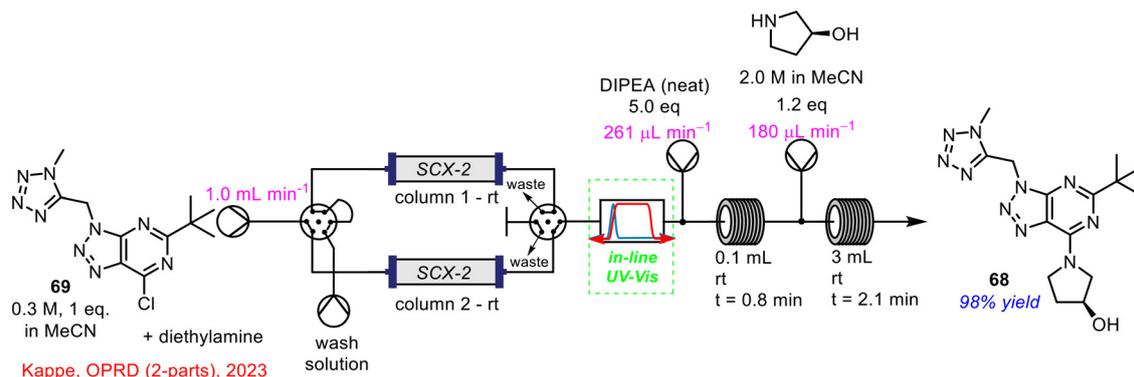
**Scheme 25** Telescoped amine scavenging with nucleophilic aromatic substitution in flow using in-line UV-vis spectrometry developed by Kappe and co-workers.<sup>67,68</sup>
