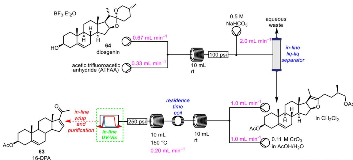
**Scheme 23** Telescoped flow synthesis of 16-DPA using in-line UV-vis spectroscopy to monitor reaction completion.<sup>61</sup>
