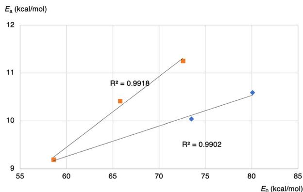
Fig. 6 Activation energy calculated using Arrhenius plot.
