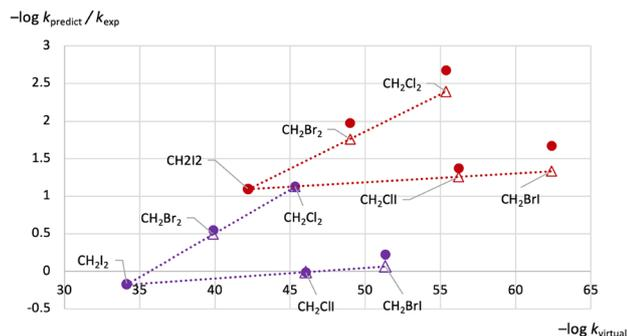
**Fig. 4** Prediction plot at different temperatures and comparison to the experimentally determined values. Circle dot: Experimental kinetic values compared to the corresponding virtual kinetic values. Outlined triangle dot: Predicted values compared to the corresponding virtual kinetic values. Red color:  $-40\text{ }^{\circ}\text{C}$ , purple color:  $0\text{ }^{\circ}\text{C}$ .
