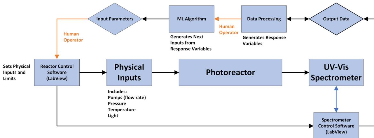
**Fig. 3** A schematic diagram of data flows in the design of experiments setup for measuring the photocatalytic degradation of an azo dye using a static mixer under continuous flow. As shown the ML algorithm of choice in this setting is a Bayesian optimisation framework which can take observed outcomes of previously performed experiments and suggest the next experiment to perform. Lines in orange indicate where intervention by a human operator is required in the current optimisation loop.
