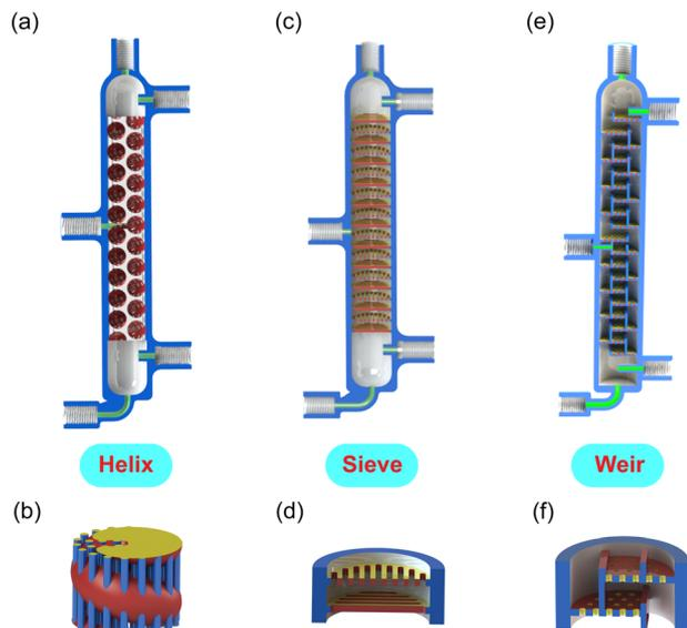
**Fig. 2** Illustration of the tray columns, *i.e.*, (a and b) helix, (c and d) sieve, and (e and f) weir structures. In order to better display the 3D structure, (b) shows the pathway through which the gas-liquid fluids flow, while (d) and (f) show half the structural units.
