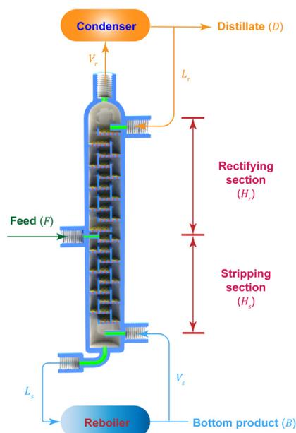
**Fig. 5** 1D mass transfer model of the microrectification geometry.**Table 4** The fitted  $k_{\text{all}}$  of all columns
