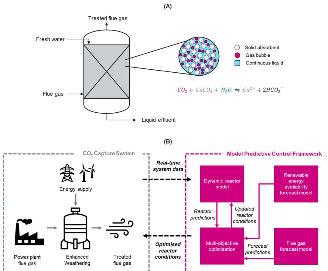
Fig. 1 Schematic representation of (A) enhanced weather packed bubble column reactor and (B) the model predictive control framework developed to maximise enhanced weathering reactor CO<sub>2</sub> capture rate, whilst simultaneously minimising non-renewable energy consumption.
