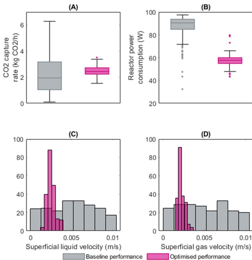
**Fig. 6** Comparing baseline and optimised performance of the enhanced weather reactors for the (A) CO<sub>2</sub> capture rate and (B) reactor power consumption, including the optimised operating conditions (C) superficial liquid velocity and (D) superficial gas velocity.
