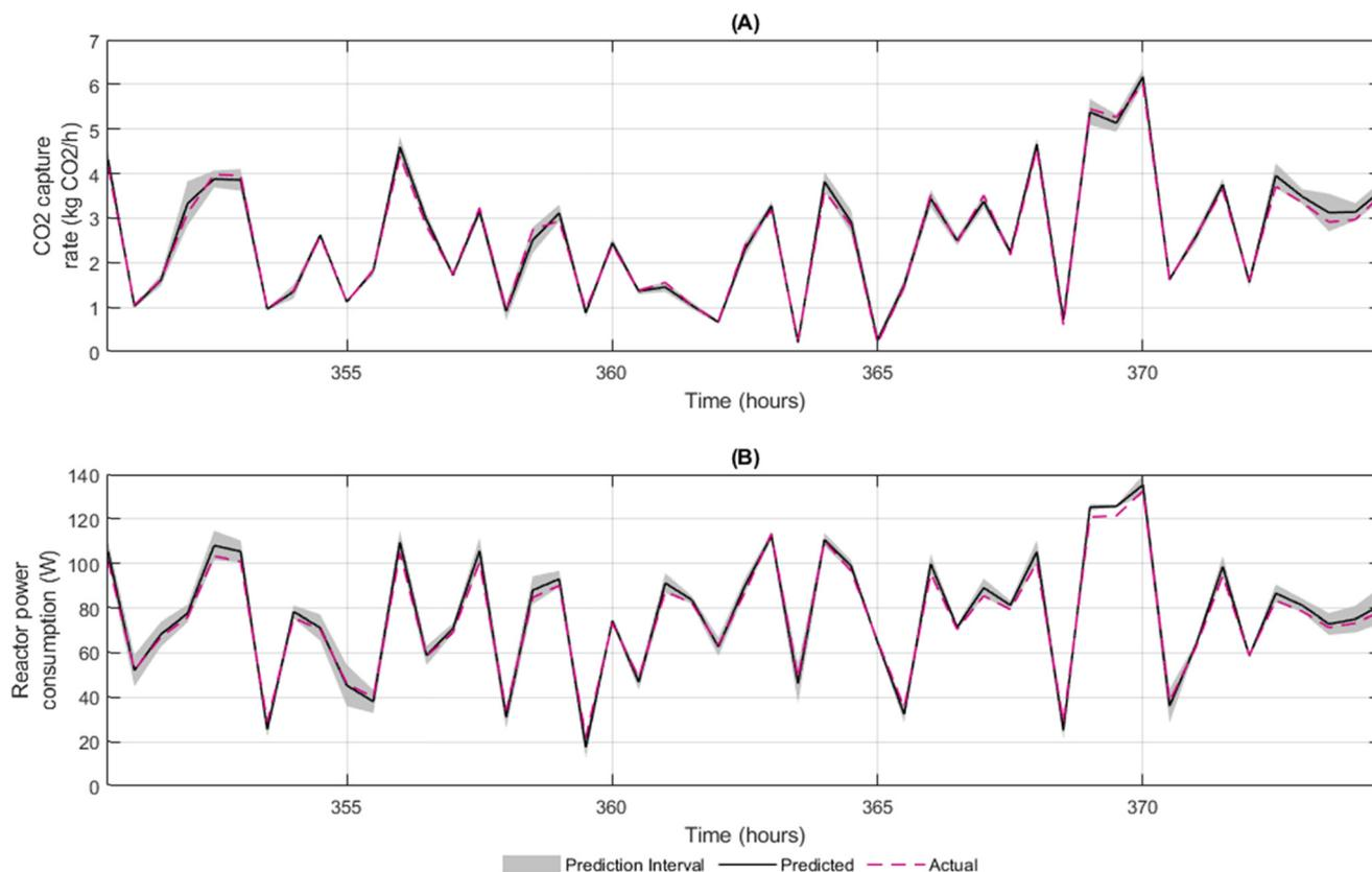
**Fig. 4** Comparison of CO<sub>2</sub> capture rate (A) and reactor power consumption (B) predictions against actual values, including prediction intervals determined using conformal prediction, over a 24-hour operation of the reactors using unseen data.
