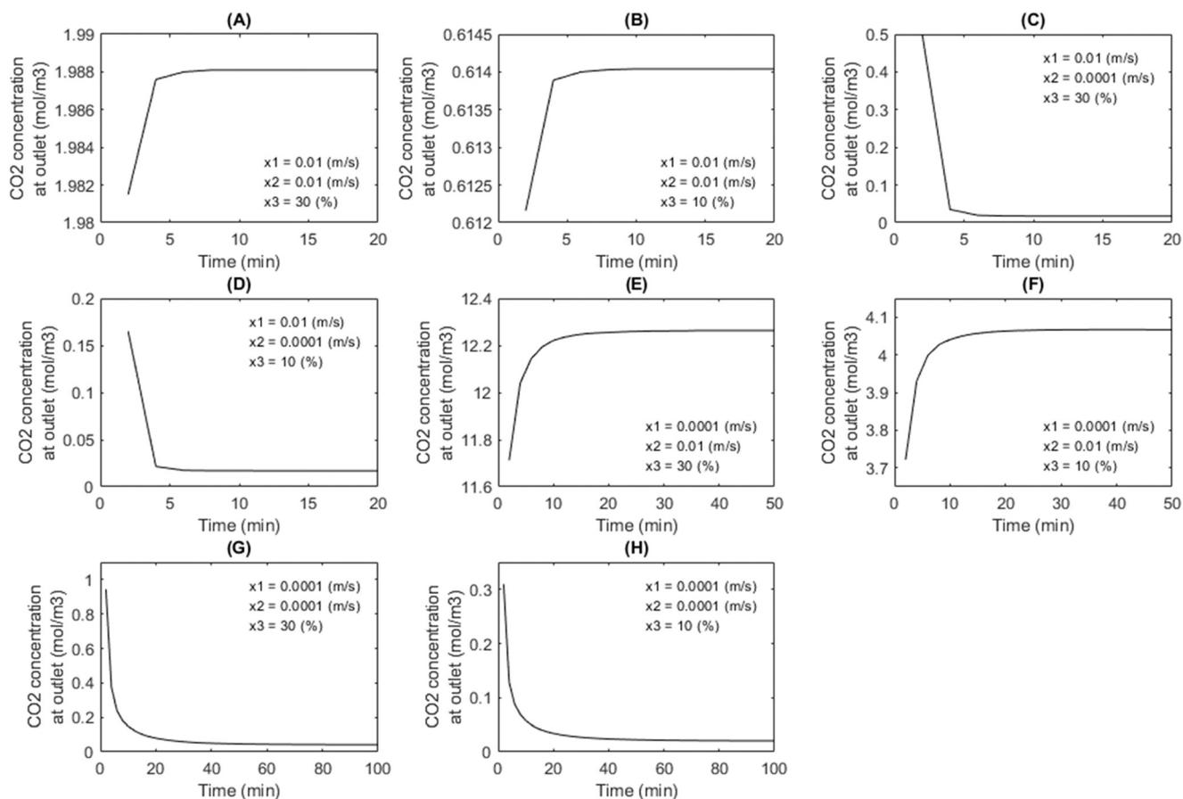
Fig. 3 Impact of reactor parameters ( $x_1$ : superficial liquid velocity;  $x_2$ : superficial gas velocity;  $x_3$  CO<sub>2</sub> inlet concentration) on time to return to equilibrium for eight scenarios (A–H) of the permutations of the maximum and minimum values of  $x_1$ ,  $x_2$  and  $x_3$ .
