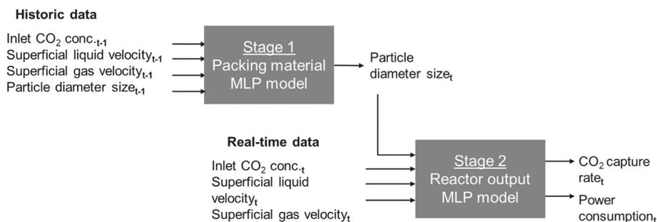
Fig. 2 The two-stage multilayer perceptron network (MLP) dynamic model to predict CO<sub>2</sub> capture rate and the power consumption of the enhanced weathering packed bubble column reactor with respect to deteriorating packing material size.
