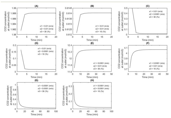
Fig. 3 Impact of reactor parameters ( $x_1$ : superficial liquid velocity;  $x_2$ : superficial gas velocity;  $x_3$  CO<sub>2</sub> inlet concentration) on time to return to equilibrium for eight scenarios (A-H) of the permutations of the maximum and minimum values of  $x_1$ ,  $x_2$  and  $x_3$ .
