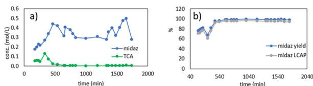
**Fig. 15** Results of 28 hour production campaign. a) Molar concentration of TCA and midazolam in dissolution outlet b) instantaneous yield and LCAP of midazolam in dissolution outlet. LCAP = liquid chromatography area percent. Midaz = midazolam.
