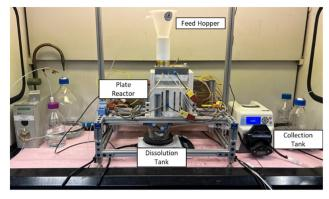
Fig. 13 Plate reactor equipment train for the production campaign.
