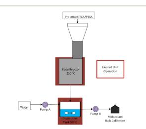
Fig. 12 Process flow diagram of the plate reactor and continuous dissolution.
