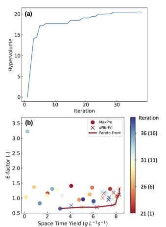
Fig. 3 Results of multi-objective optimisation of the Schotten-Baumann reaction. (a) Hypervolume improvement versus iteration number. (b) Optimisation results and the Pareto front (the colorbar represents the sequence of the iteration step from 1-20 for the initial design and 21-39 for the optimisation results).
