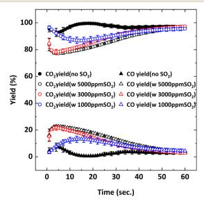
Fig. 5 CO<sub>2</sub> and CO yields as a function of reduction period during the 5th cycle at 900 °C with 9% CH<sub>4</sub>-X ppm SO<sub>2</sub>-balance N<sub>2</sub> where X: 0, 1000, 3000, 5000.
