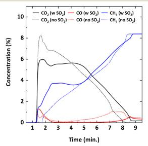
Fig. 6 Flue gas concentration profiles during complete reduction of Cu34Mn66 particles at 900  $^{\circ}$ C with 9% CH<sub>4</sub>-balance N<sub>2</sub> and 9% CH<sub>4</sub>-5000 ppm SO<sub>2</sub>-balance N<sub>2</sub>.
