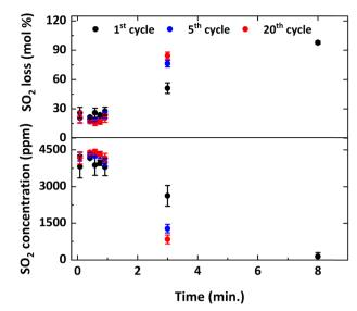
Fig. 7 Measured  $SO_2$  concentration profile and calculated  $SO_2$  loss (mol%) as a function of reduction period for the 1st, 5th, and 20th cycles at 900 °C with 9%  $CH_4$ -5000 ppm  $SO_2$ -balance  $N_2$ .
