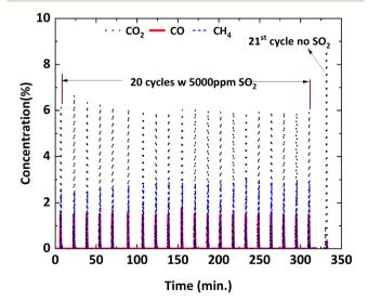
Fig. 14 Multicycle redox behavior of Cu34Mn66 particles at 900 °C with 9% CH<sub>4</sub>-5000 ppm SO<sub>2</sub>-balance N<sub>2</sub>. Reducing time is 1 minute.
