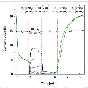
Fig. 3 Flue gas concentration profiles during the 5th cycle at 900 °C with and without 5000 ppm SO<sub>2</sub>. The reducing gas is 9% CH<sub>4</sub>-balance  $N_2$  and 9%  $CH_4$ -5000 ppm  $SO_2$ -balance  $N_2$ . The oxidizing gas is air.
