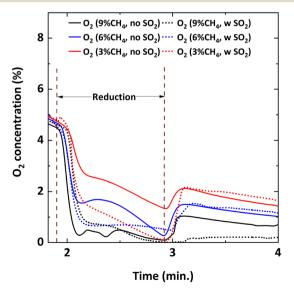
Fig. 10 O<sub>2</sub> concentration profile during the 5th cycle at 900 °C with Y% CH<sub>4</sub>-balance N<sub>2</sub> and Y% CH<sub>4</sub>-5000 ppm SO<sub>2</sub>-balance N<sub>2</sub> where Y: 3, 6, 9.
