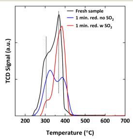
Fig. 20 H<sub>2</sub>-TPR spectra of fresh Cu34Mn66 and samples reduced for 1 minute for 5 cycles at 900 °C with 9% CH<sub>4</sub>-balance N<sub>2</sub> and 9% CH<sub>4</sub>-5000 ppm SO<sub>2</sub>-balance N<sub>2</sub>.
