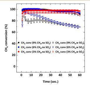
Fig. 8 CH<sub>4</sub> conversion as a function of reduction period during the 5th cycle at 900  $^{\circ}$ C with Y% CH<sub>4</sub>-balance N<sub>2</sub> and Y% CH<sub>4</sub>-5000 ppm SO<sub>2</sub>-balance N<sub>2</sub> where Y: 3, 6, 9.
