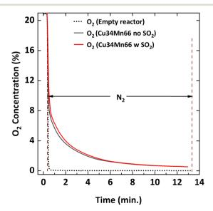
Fig. 2 O<sub>2</sub> concentration profile during oxygen uncoupling of Cu34Mn66 particles in N<sub>2</sub> at 900 °C with and without 5000 ppm SO<sub>2</sub>.
