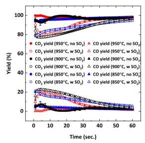
Fig. 12 CO<sub>2</sub> and CO yields as a function of reduction period during the 5th cycle with 9%  $CH_4$ -balance  $N_2$  and 9%  $CH_4$ -5000 ppm  $SO_2$ balance N<sub>2</sub> at different temperatures (850, 900, 950 °C).
