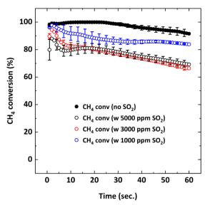
Fig. 4 CH<sub>4</sub> conversion as a function of reduction period during the 5th cycle at 900 °C with 9% CH<sub>4</sub>-X ppm SO<sub>2</sub>-balance N<sub>2</sub> where X: 0, 1000, 3000, 5000
