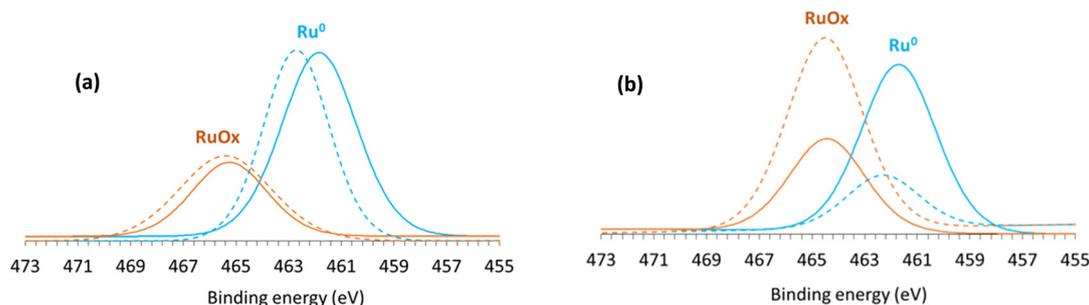
Fig. 7 XPS results for (a) Ru<sup>R</sup>/IC-1 (continuous line) and Ru/IC-1 (dotted line), and (b) Ru<sup>R</sup>/SA-30 (continuous line) and Ru/SA-30 (dotted line). Signals in orange and blue correspond to RuO<sub>x</sub> and Ru(0), respectively.
