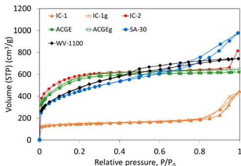
Fig. 3 N<sub>2</sub> adsorption-desorption isotherms at -196 °C for the carbon supports.
