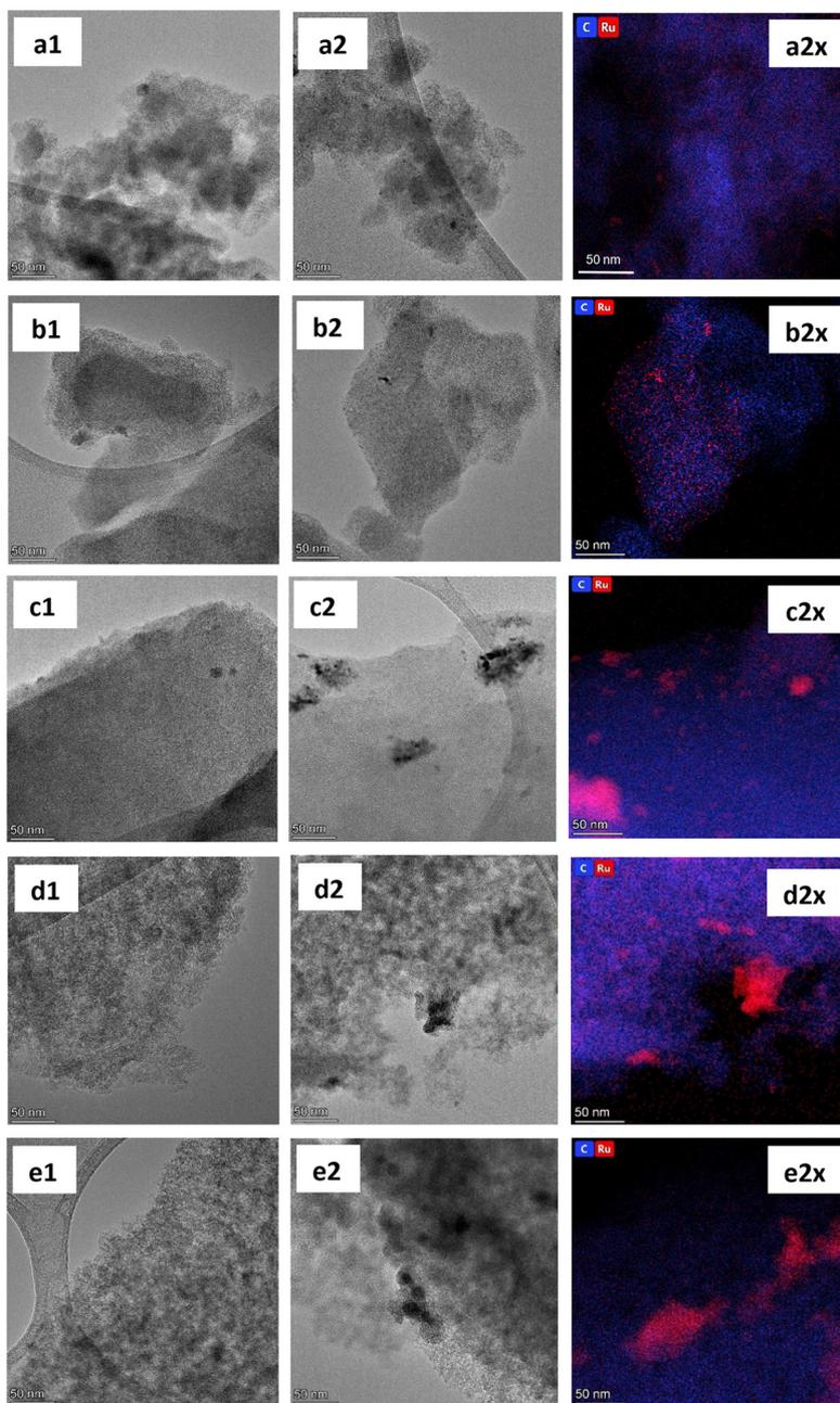
**Fig. 6** TEM images of un-reduced and reduced catalysts and EDX of reduced catalysts: Ru/IC-1 (a1), Ru<sup>R</sup>/IC-1 (a2 and a2x), Ru/IC-2 (b1), Ru<sup>R</sup>/IC-2 (b2 and b2x), Ru/ACGE (c1), Ru<sup>R</sup>/ACGE (c2 and c2x), Ru/SA-30 (d1), Ru<sup>R</sup>/SA-30 (d2 and d2x), Ru<sup>R</sup>/WV-1100 (e1) and Ru<sup>R</sup>/WV-1100 (e2 and e2x). Images have been obtained with the TALOS F200X Microscope coupled to an EDX system.
