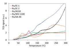
Fig. 5 TPR profiles of the Ru/C samples.
