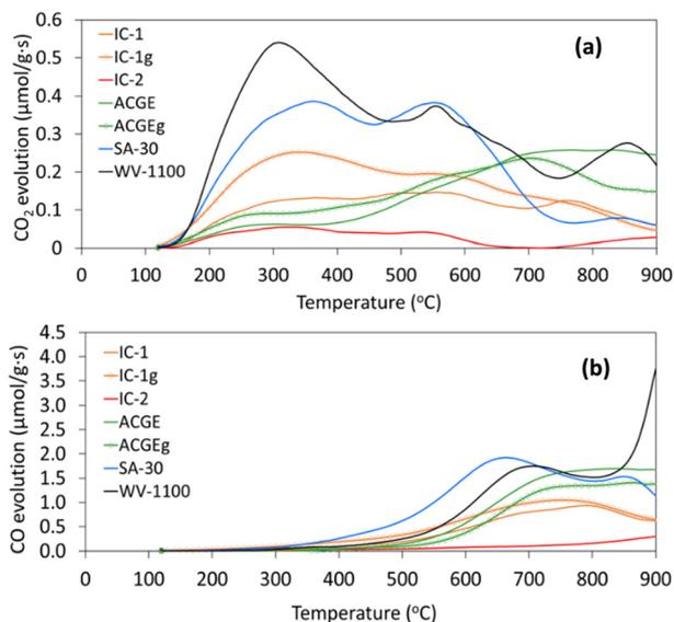
Fig. 4 TPD spectra of supports and reduced catalysts: evolution of (a)  $\text{CO}_2$  and (b)  $\text{CO}$ . (be aware of the different y-axis scale in figures (a) and (b)).
