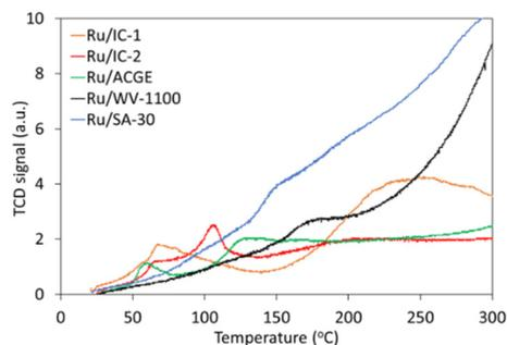
Fig. 5 TPR profiles of the Ru/C samples.
