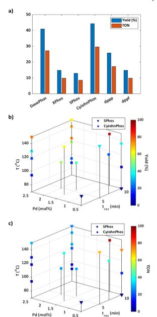
Fig. 2 Suzuki-Miyaura self-optimisation results: a) responses for the six centre point initialisation experiments; b) reaction profile with respect to the yield of 3; c) reaction profile with respect to catalyst TON.
