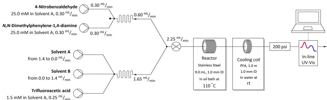
Fig. 5 Flow setup and reaction conditions used in solvents mixtures studies in imine formation reaction.
