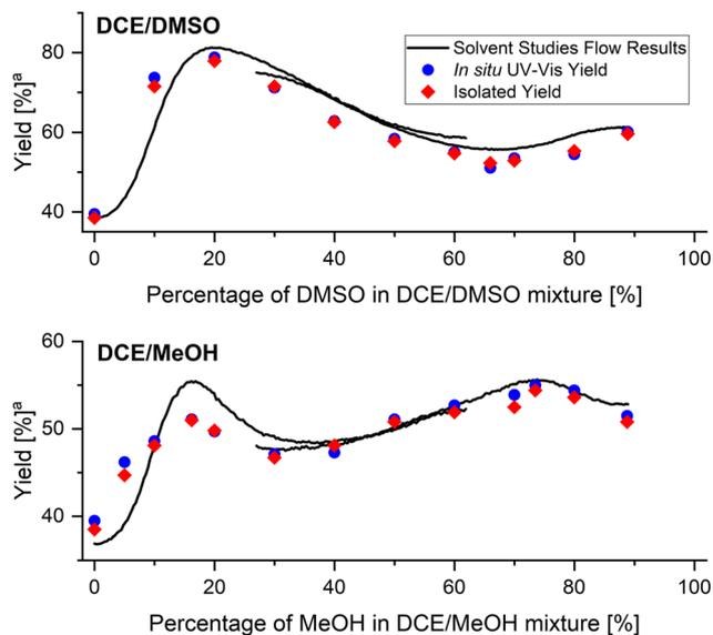
Fig. 7 Comparison of flow and validation results of imine formation reaction. <sup>a</sup>Yield at fixed residence time of 240 seconds.
