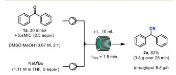
Scheme 3 Reaction scalability demonstrated on 30 mmol scale
