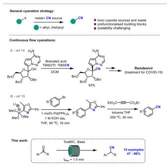
**Scheme 1** Overview of different batch and flow-based cyanation processes. A: A large-scale continuous flow cyanation process towards Remdesivir. B: A cyanide-free cyanation in batch mode using an oxazole-based masked nitrile source.
