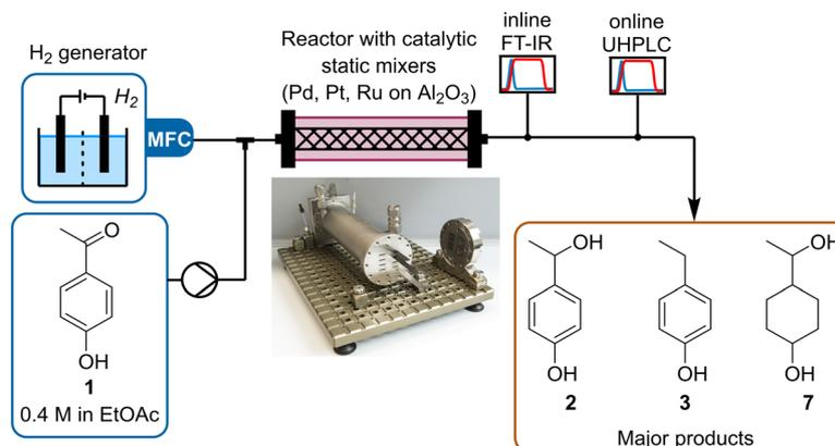
Fig. 1 Schematic representation of the setup used to study the hydrogenation of ketone **1**, using different metal/Al<sub>2</sub>O<sub>3</sub> CSMs.
