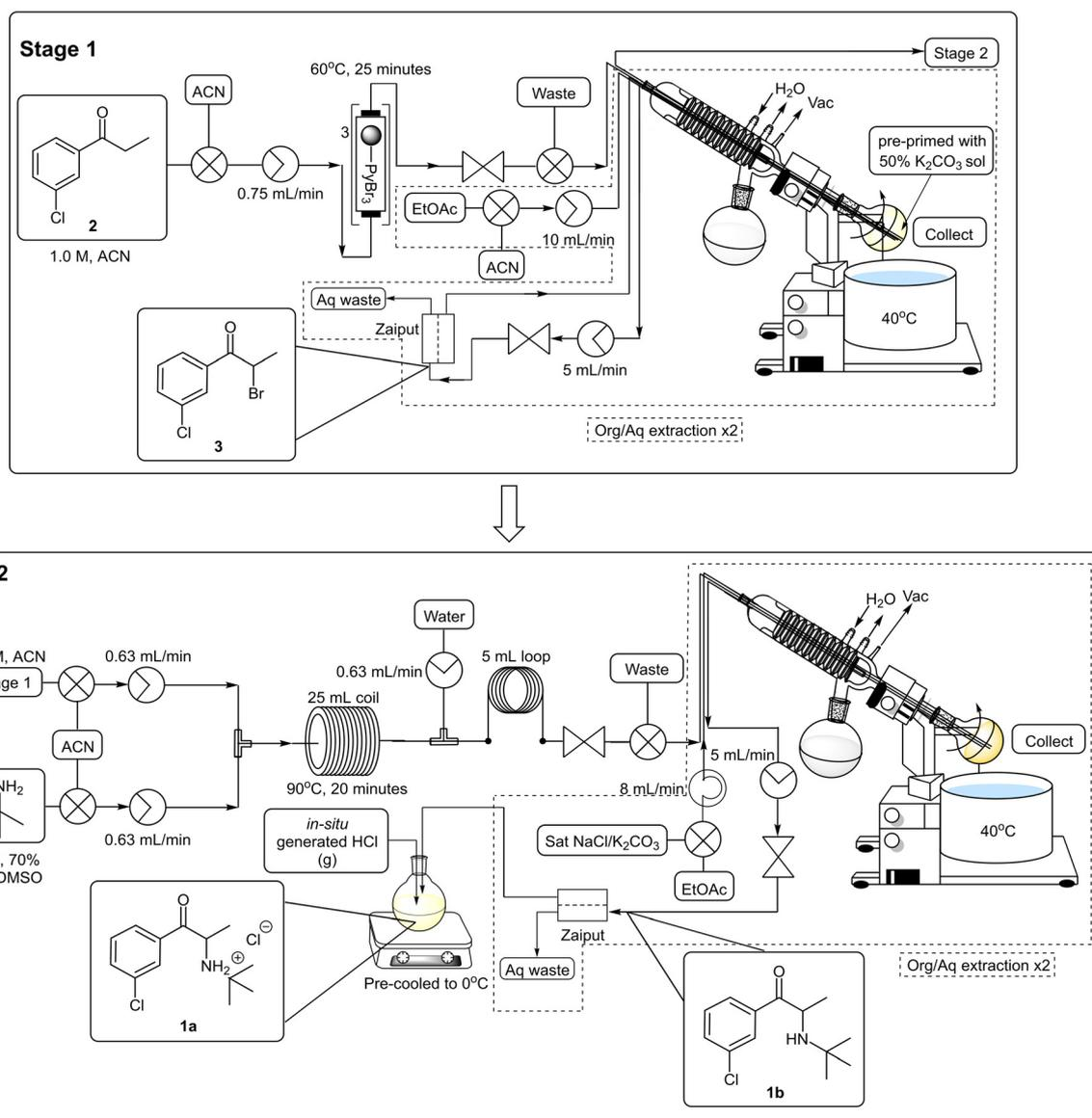
Scheme 8 4th generation flow synthesis of bupropion hydrochloride **1a**.
