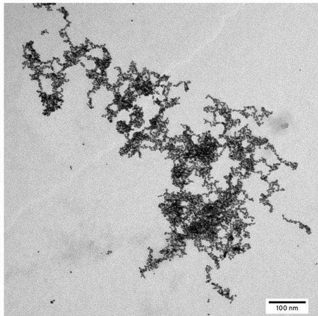
Fig. 4 TEM images of Au NPs synthesized in jet-mixing with 0.90 mM  $\text{NaBH}_4$  and 0.27 mM  $\text{HAuCl}_4$  in absence of stabilizing ligand. The main line and jet line flowrates in the single jet-mixer are maintained at  $48 \text{ mL h}^{-1}$ .
