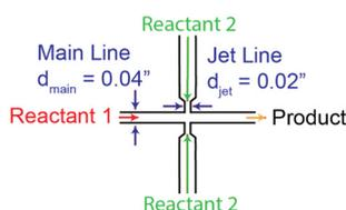
**Fig. 1** Geometry of a jet-mixing reactor (JMR) unit with a main line ( $d_{\text{main}} = 0.04''$ ;  $1000 \mu\text{m}$ ) carrying reactant 1 and an orthogonally impinging jet line ( $d_{\text{jet}} = 0.02''$ ;  $500 \mu\text{m}$ ) consisting of a pair of jets carrying reactant 2. The product is collected downstream of the reactor.
