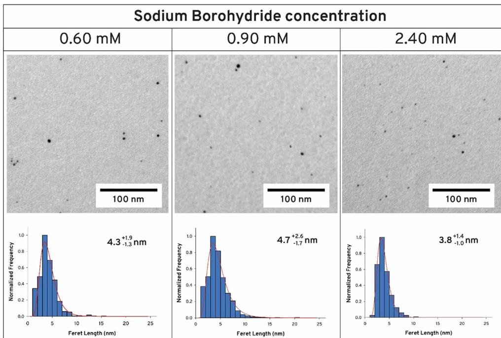
Fig. 6 TEM images of Au NPs synthesized via jet mixing reactor at 0.27 mM HAuCl<sub>4</sub> and different concentrations of NaBH<sub>4</sub> with post-synthesis addition of a cold BSA aqueous solution.
