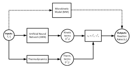
Fig. 2 Pathway from inputs to outputs for the microkinetic model (MKM) (dashed lines) and the proposed artificial neural network (ANN) (solid lines).
