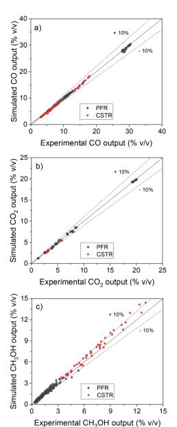
Fig. 10 Validation of the ANN<sub>30</sub> with steady-state experimental data performed in a PFR<sup>10</sup> and in a CSTR.<sup>18</sup> (a) CO. (b) CO<sub>2</sub>. (c) CH<sub>3</sub>OH.
