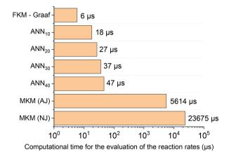
Fig. 11 Average computational time of different models to calculate the reaction rates ( $\mu$ s). FKM – Graaf refers to the formal kinetic model developed by Graaf et al.<sup>24</sup> The microkinetic model was solved by two approaches: providing the analytical Jacobian matrix (AJ) and calculating the Jacobian matrix numerically (NJ).
