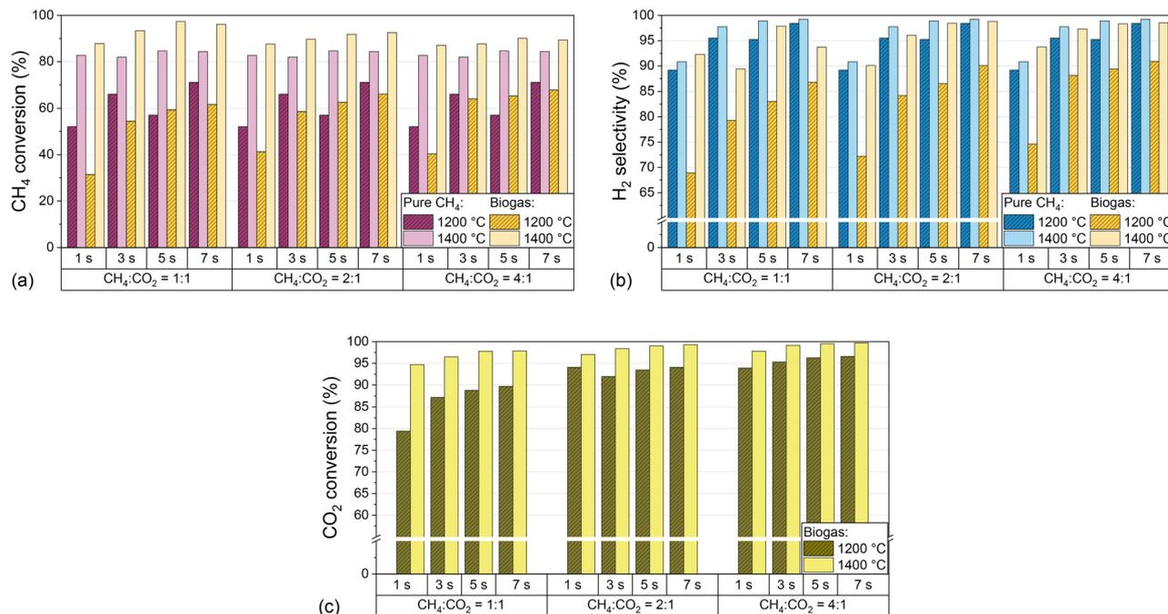
Fig. 3 Molar CH<sub>4</sub> conversion (a), molar H<sub>2</sub> selectivity (b), and molar CO<sub>2</sub> conversion (c) as a function of residence time and CH<sub>4</sub>:CO<sub>2</sub> ratio of biogas at 1200 °C to 1400 °C, and a molar H<sub>2</sub>:biogas ratio of 2:1. As reference, data obtained with a feed gas that contains only CH<sub>4</sub> (in H<sub>2</sub> as a dilutant with a molar H<sub>2</sub>:CH<sub>4</sub> ratio of 2:1) are also plotted in (a) and (b).
