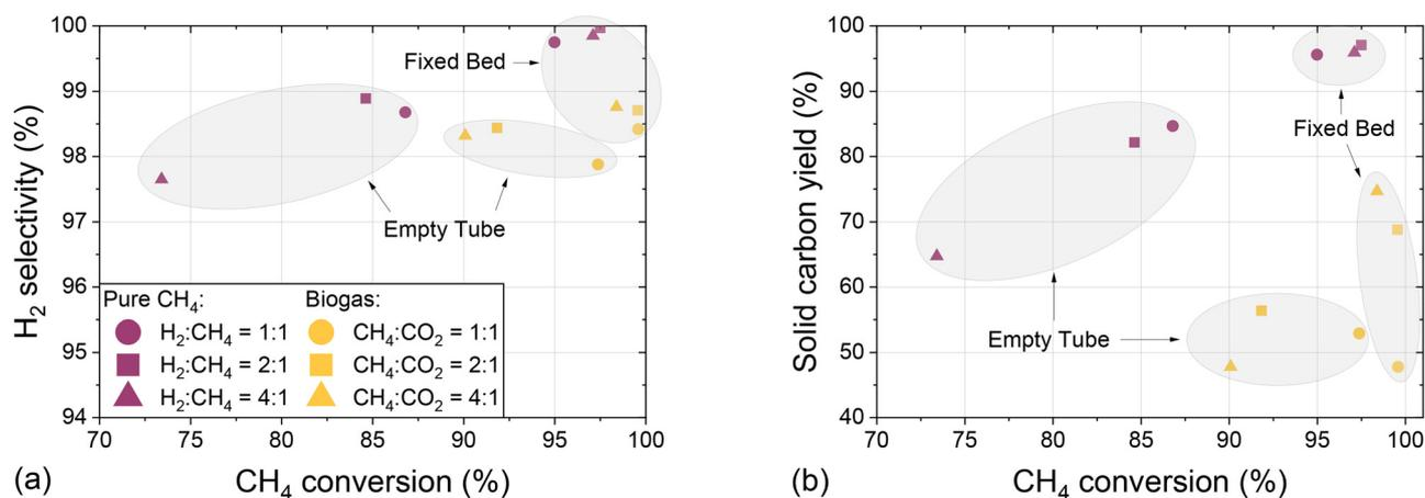
Fig. 8 Molar  $\text{H}_2$  selectivity (a) and mass-based solid carbon yield (b) as a function of molar  $\text{CH}_4$  conversion for pure  $\text{CH}_4$  and biogas feeds in an empty tube and fixed bed configuration at a temperature of 1400 °C, a residence time of 5 s, and a constant molar  $\text{H}_2$ :biogas ratio of 2:1.
