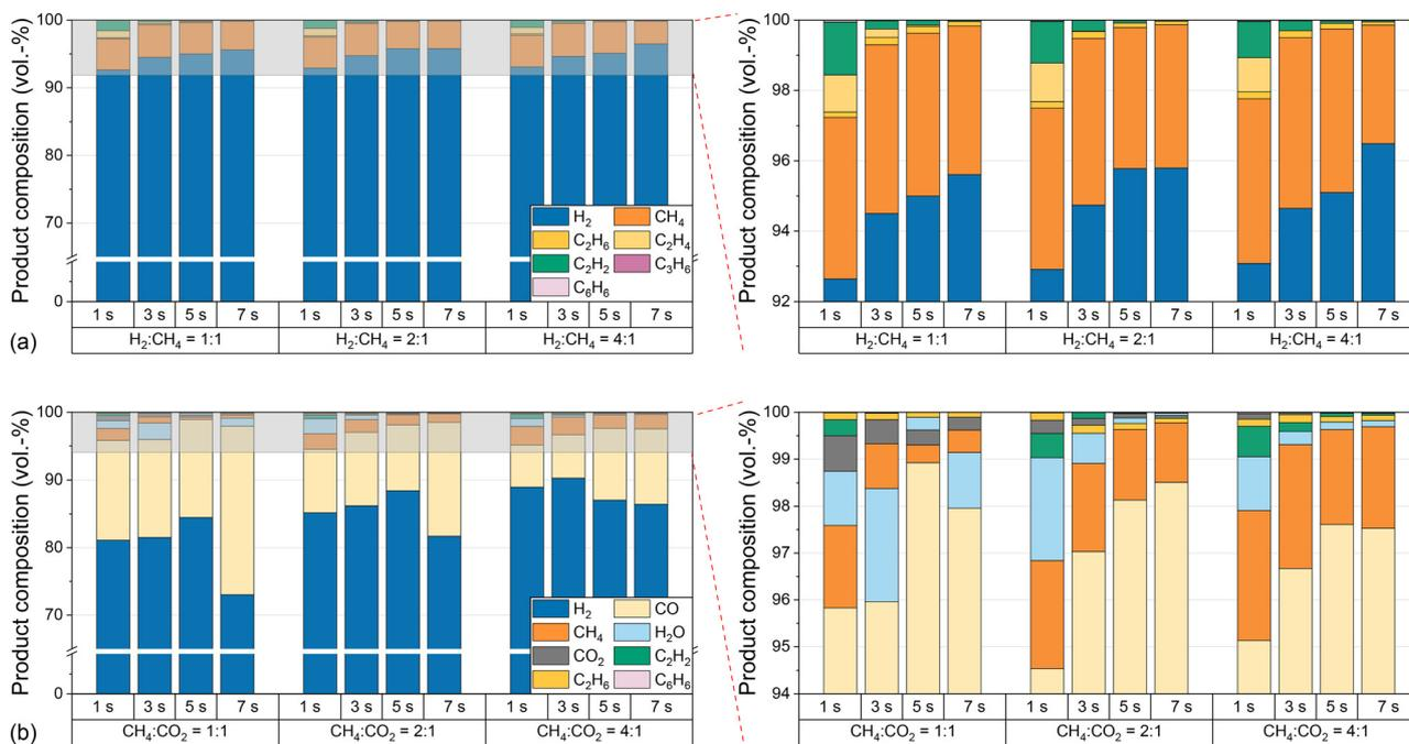
Fig. 4 Product composition for pure CH<sub>4</sub> (a) and biogas (b) as a function of residence time, molar H<sub>2</sub>:CH<sub>4</sub> dilution, and molar CH<sub>4</sub>:CO<sub>2</sub> ratio of biogas (in H<sub>2</sub> as a dilutant with a molar H<sub>2</sub>:biogas ratio of 2:1) at 1400 °C.
