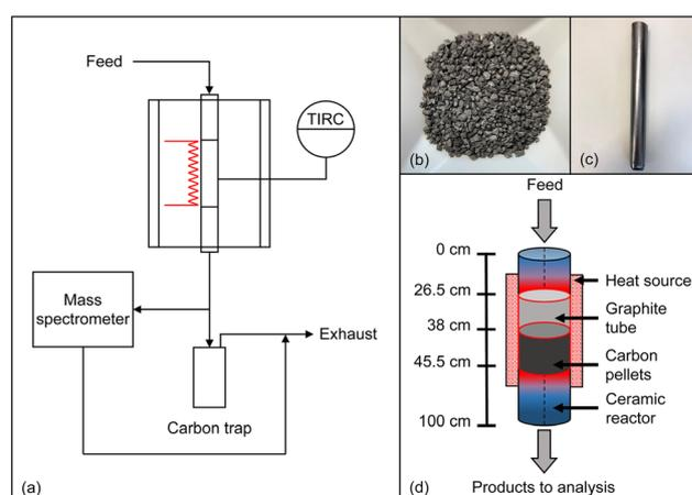
**Fig. 1** Schematic flow diagram of the experimental setup (a), acetylene coke used as a base material of the fixed bed (b), a graphite container with flow holes at the bottom (c), and a scheme of the positioning of the carbon fixed bed container in the reactor (d).
