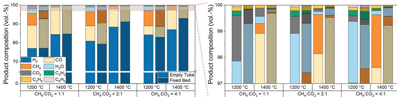
Fig. 7 Empty tube and fixed bed results for product composition for biogas as a function of temperature and molar  $\text{CH}_4:\text{CO}_2$  ratio of biogas at a constant residence time of 5 s and a molar  $\text{H}_2$  dilution ratio of 2:1.
