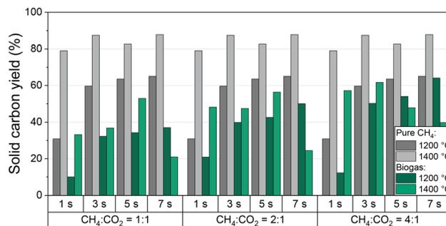
Fig. 5 Mass-based solid carbon yield as a function of residence time and molar  $\text{CH}_4$ : $\text{CO}_2$  ratio of biogas at 1200 °C to 1400 °C, and a molar  $\text{H}_2$ :biogas ratio of 2:1. As reference, data obtained with a feed gas that contains only  $\text{CH}_4$  (in  $\text{H}_2$  as a dilutant with a molar  $\text{H}_2$ : $\text{CH}_4$  ratio of 2:1) is also plotted.
