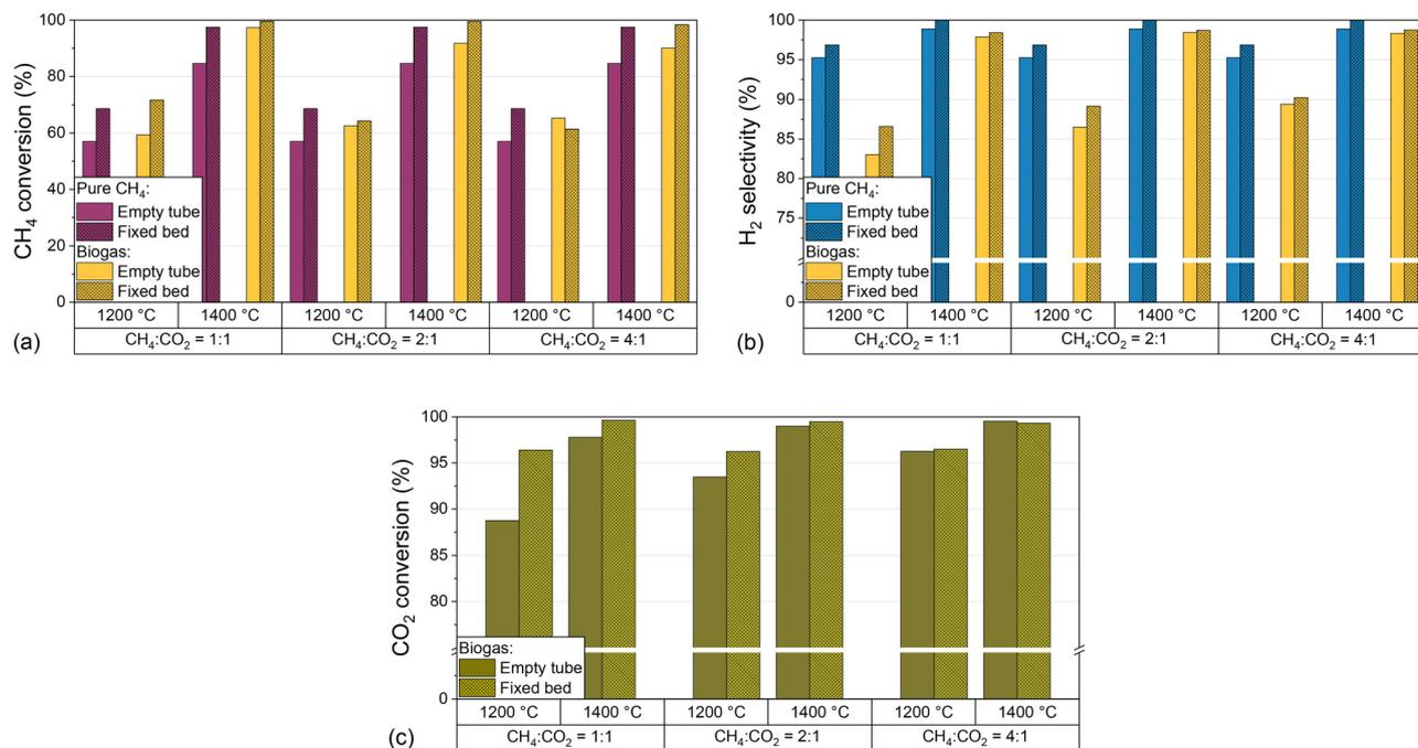
Fig. 6 Empty tube and fixed bed results for molar CH<sub>4</sub> conversion (a), molar H<sub>2</sub> selectivity (b) for pure CH<sub>4</sub> and biogas and molar CO<sub>2</sub> conversion (c) for biogas as a function of temperature and molar CH<sub>4</sub>:CO<sub>2</sub> ratio of biogas at a constant residence time of 5 s and a molar H<sub>2</sub> dilution ratio of 2:1.
