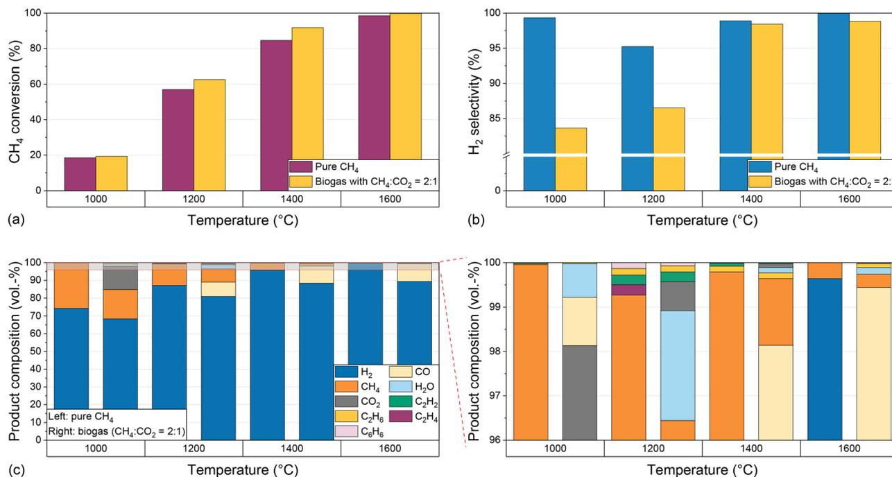
Fig. 2 Molar CH<sub>4</sub> conversion (a), molar H<sub>2</sub> selectivity (b), and product composition (c) for pure CH<sub>4</sub> and biogas (CH<sub>4</sub>:CO<sub>2</sub> ratio 2:1) as a feed at temperatures from 1000 °C to 1600 °C, a residence time of 5 s, a molar H<sub>2</sub>:CH<sub>4</sub> ratio of 2:1, and a molar H<sub>2</sub>:biogas ratio of 2:1.
