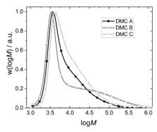
Fig. 5 Exemplary molecular weight distributions of the final PPG products of pulse experiments with DMC A-C.
