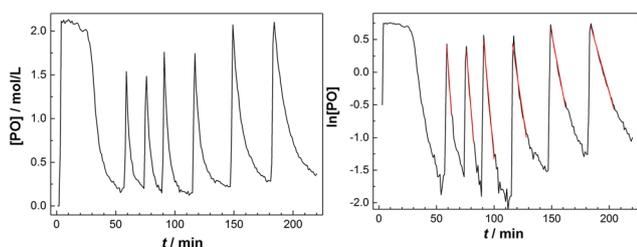
Fig. 2 The concentration of PO decreases exponentially with reaction time  $t$  (left), linearization allows determination of rate coefficients  $k_{\text{obs}}$  from the slope of the fit in the initial phase (right).
