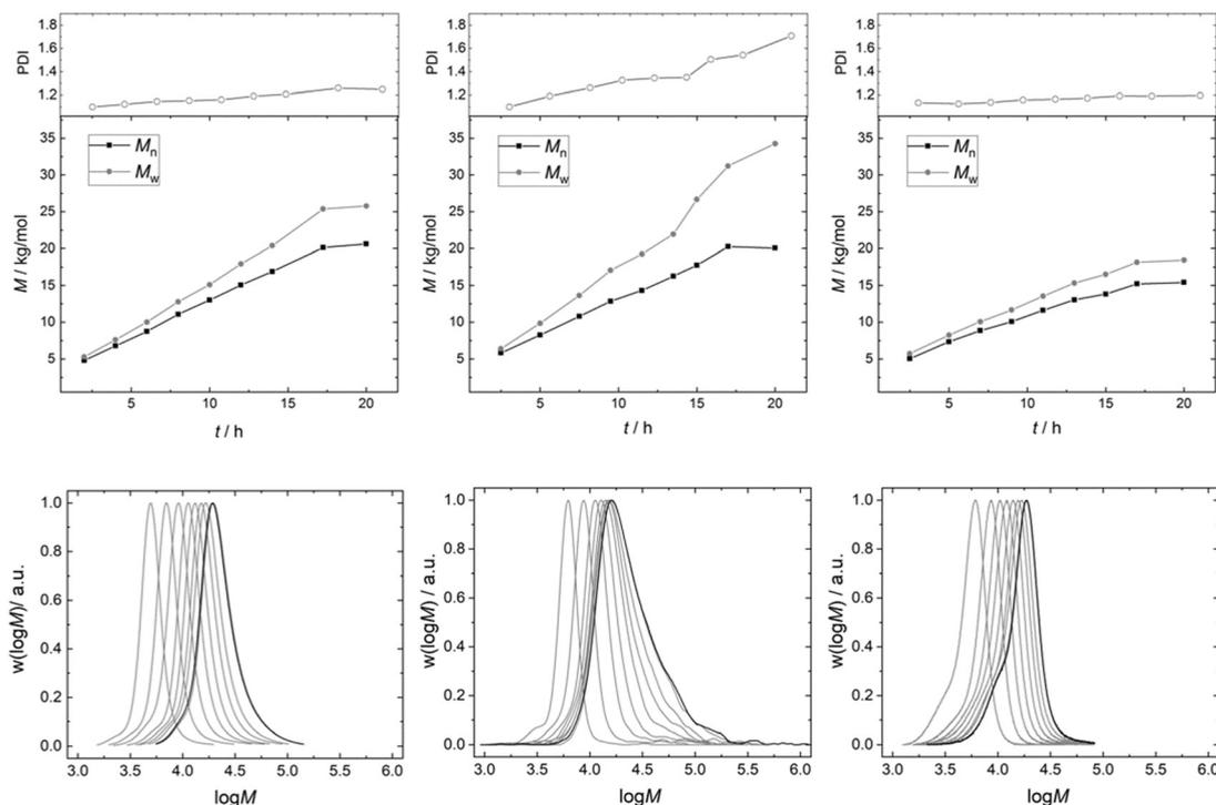
Fig. 7 SEC-analysis of PPGs synthesized by PO homopolymerization with 50 mg of DMC A (l), 50 mg of DMC B (m) and 450 mg of DMC B (r), with number average ( $M_n$ ) (black) and weight average ( $M_w$ ) (grey) molecular weights of PPGs synthesized by propoxylation.
