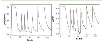
Fig. 2 The concentration of PO decreases exponentially with reaction time t (left), linearization allows determination of rate coefficients  $k_{\rm obs}$ from the slope of the fit in the initial phase (right).
