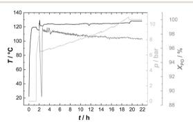
Fig. 6 Temperature and pressure profiles and conversion of PO during the semi-batch process with DMC A (PO was dosed to the nonactivated catalyst after about 2 h, giving a spike of PO, which disappeared, showing that the catalyst had become active. PO semibatch feeding started after about 3 h).
