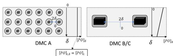
**Scheme 4** Illustration of the consequences of catalyst particle distances  $\delta$  in the propoxylation: PPGs inside the range of self-diffusion given by the rate of propoxylation are growing predominantly; more PPGs are outside the range when using larger DMC particles, leading to bimodal distributions. On the right of each case, the concentration of PO is shown as a function of  $\delta$ .
