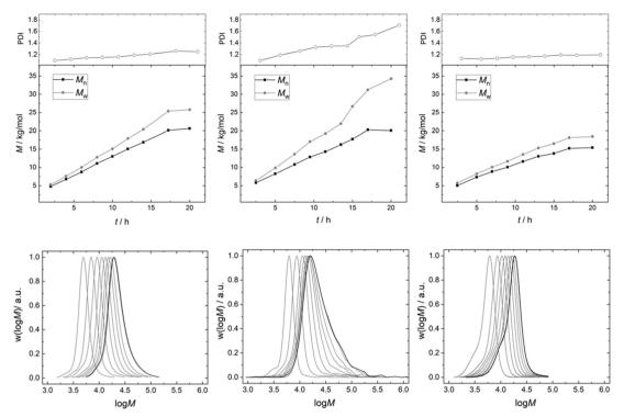
Fig. 7 SEC-analysis of PPGs synthesized by PO homopolymerization with 50 mg of DMC A (I), 50 mg of DMC B (m) and 450 mg of DMC B (r), with number average  $(M_n)$  (black) and weight average  $(M_w)$  (grey) molecular weights of PPGs synthesized by propoxylation.
