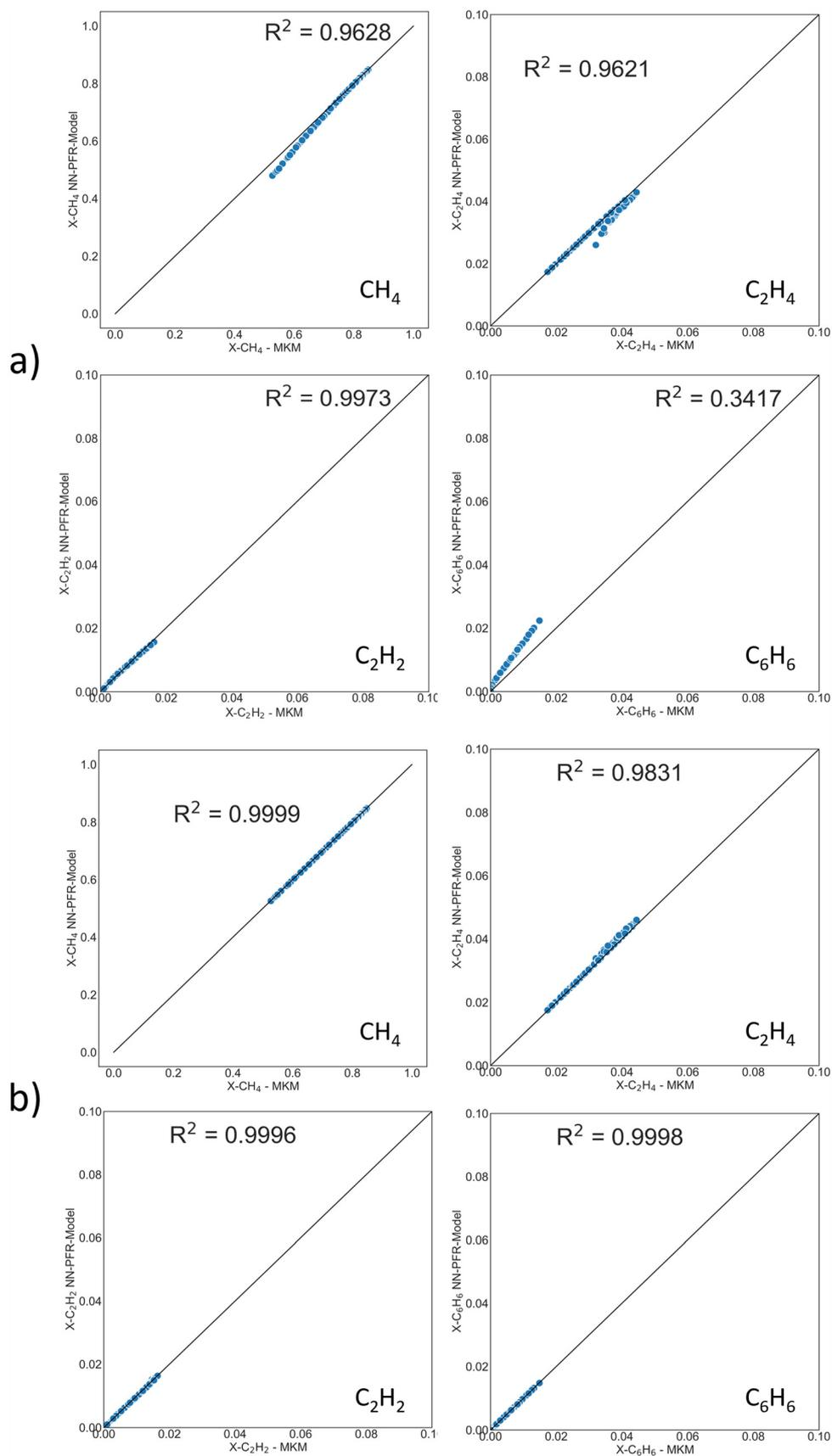
Fig. 5 Parity plots of PFR exit mole fraction of CH<sub>4</sub>, C<sub>2</sub>H<sub>4</sub>, C<sub>2</sub>H<sub>2</sub>, C<sub>6</sub>H<sub>6</sub> from DNN-based surrogate model (y-axis) and MKM (x-axis) for a) reaction set A and b) reaction set B. Trace reactions are considered for both reaction sets.
