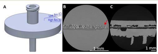
Fig. 3 A) CAD diagram with planes showing where CT images were taken from; B) a high resolution and C) low resolution CT scan showing the membrane conformally bonded to the extruded plastic on one side. The red arrow indicates a singular membrane fibre having been incorporated within the plastic.
