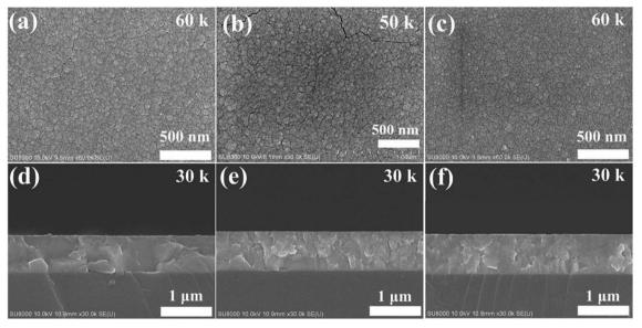
Fig. 1 Surface SEM images for (a) OSiW, (b) 6SiW and (c) 11SiW. Cross-sectional SEM images for (d) OSiW, (e) 6SiW and (f) 11SiW.
