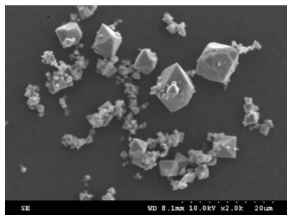
**Fig. 11(a)** SEM image for solid precipitate at 120 °C – H<sub>2</sub>O control group.
