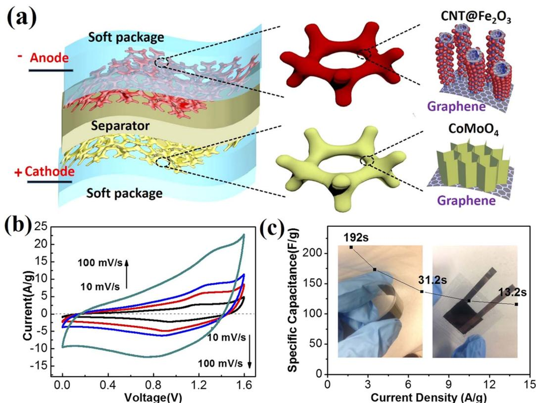
Fig. 3 Electrochemical behavior of the GF-CNT/Fe<sub>2</sub>O<sub>3</sub>//GF-CoMoO<sub>4</sub> full cell. (a) Schematic of the full-cell package. (b) CV curves, (c) rate capability.
