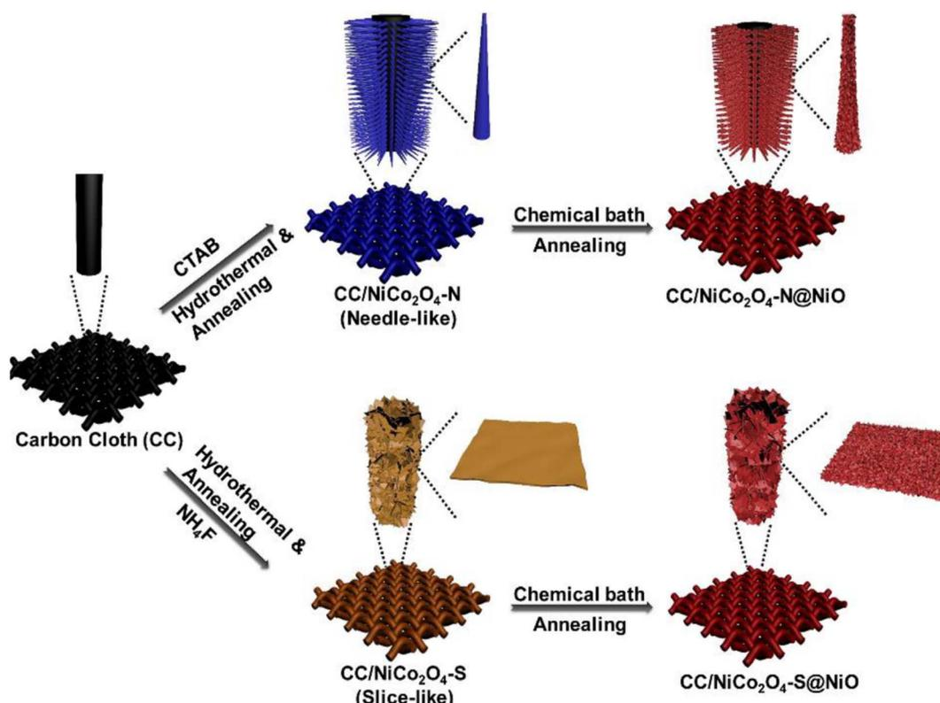
Fig. 2 Schematic of the preparation of CC/NiCo<sub>2</sub>O<sub>4</sub>-N@NiO and CC/NiCo<sub>2</sub>O<sub>4</sub>-S@NiO.<sup>133</sup>
