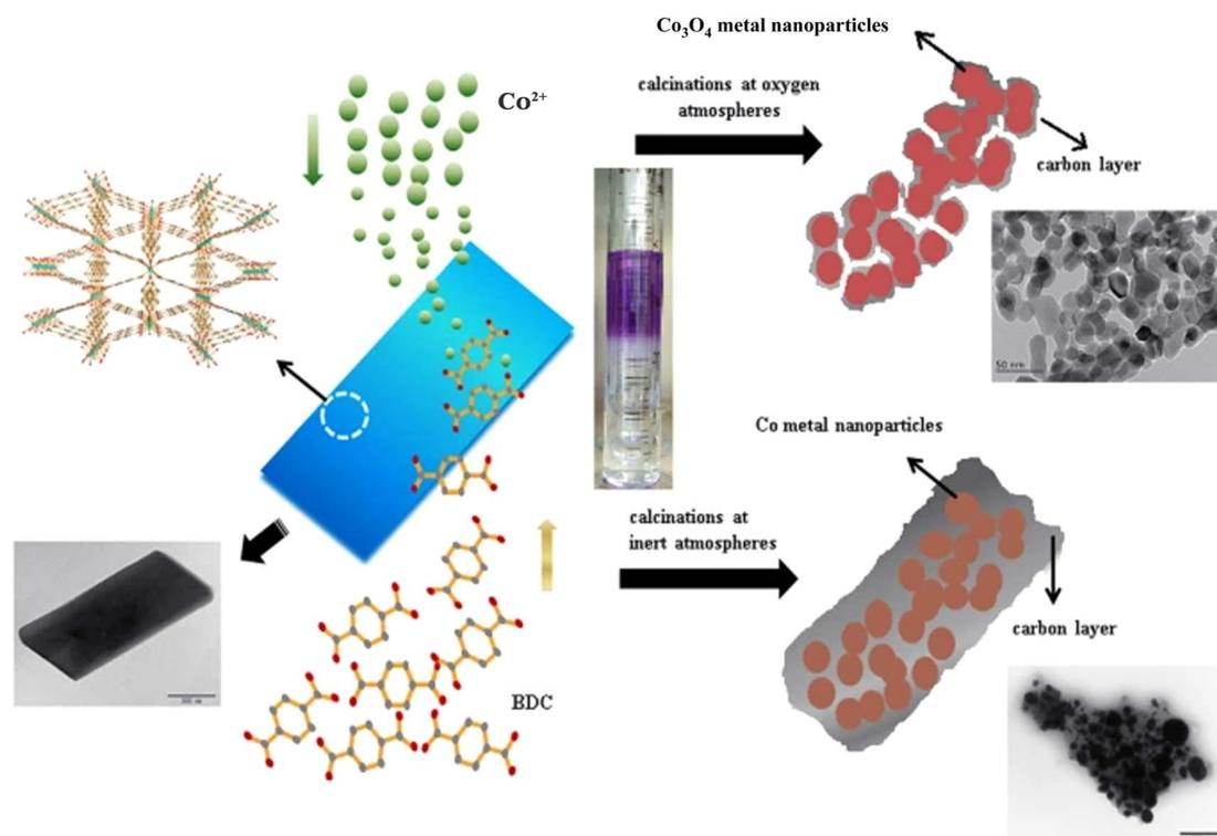
Fig. 7 Schematic of the syntheses of Co-BDC nanosheets and cobalt–carbon composites.<sup>191</sup>
