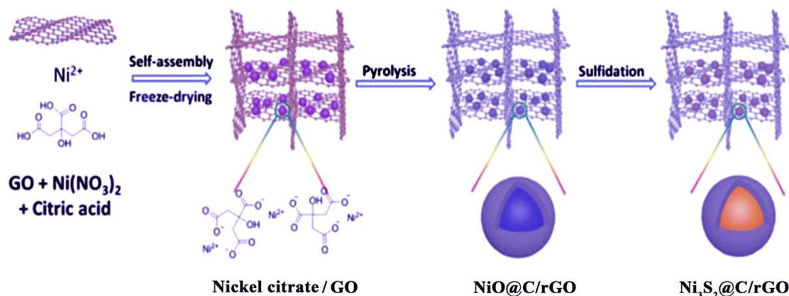
Fig. 4 Schematic of the synthesis of dual carbon-modified  $\text{Ni}_3\text{S}_2\text{-C/rGO}$ .<sup>152</sup>
