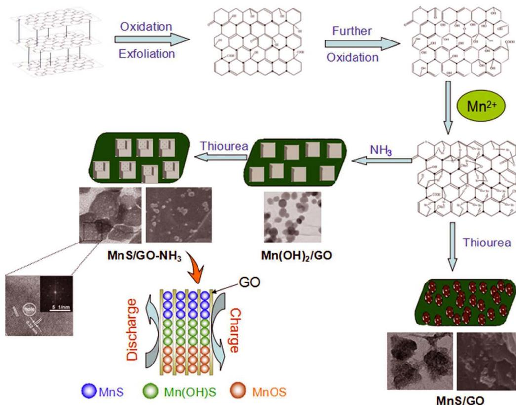
Fig. 5 Schematic of the preparation processes of MnS/GO-NH<sub>3</sub> and MnS/GO composites.<sup>156</sup>
