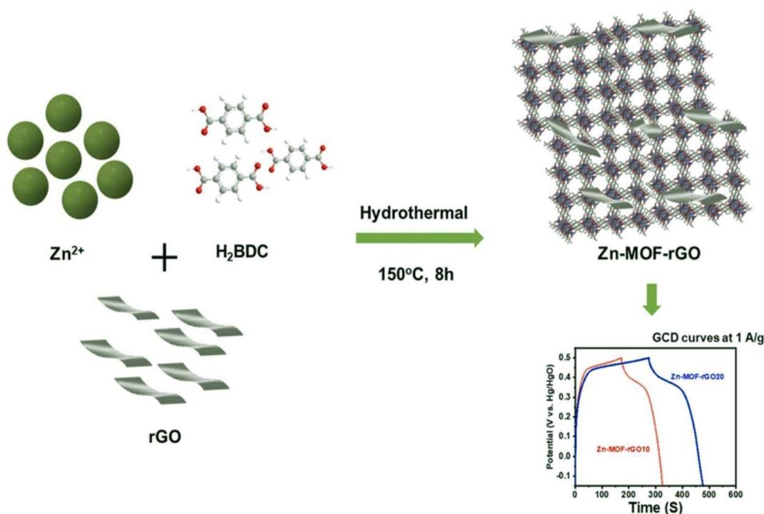
Fig. 6 Schematic of the synthesis of Zn-MOF-rGO.<sup>183</sup>
