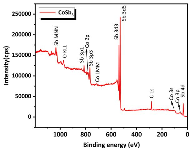
Fig. 6 Survey scan XPS spectra of CoSb<sub>3</sub>.
