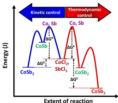
Scheme 2 Energy profile diagram for the formation of CoSb<sub>2</sub> and CoSb<sub>3</sub>.
