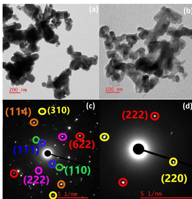
Fig. 16 (a and b) TEM images of the particles with different morphologies in the TGA residue from room temperature to 700 °C in a N<sub>2</sub> atmosphere and (c and d) SAED pattern.
