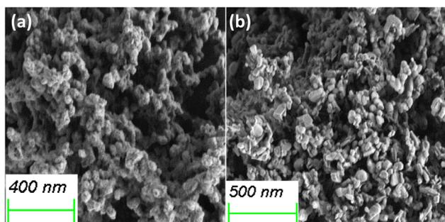
Fig. 14 SEM images of the (a) TGA residue from room temperature to 700 °C in air and (b) N<sub>2</sub> atmosphere.
