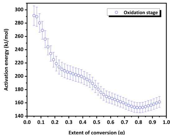
Fig. 10 Extent of conversion *versus* activation energy curve of the CoSb<sub>3</sub> oxidation stage.
