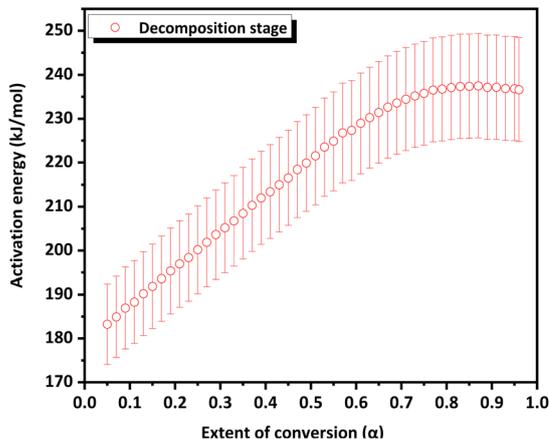
Fig. 11 Extent of conversion *versus* activation energy curve of the CoSb<sub>3</sub> decomposition stage.
