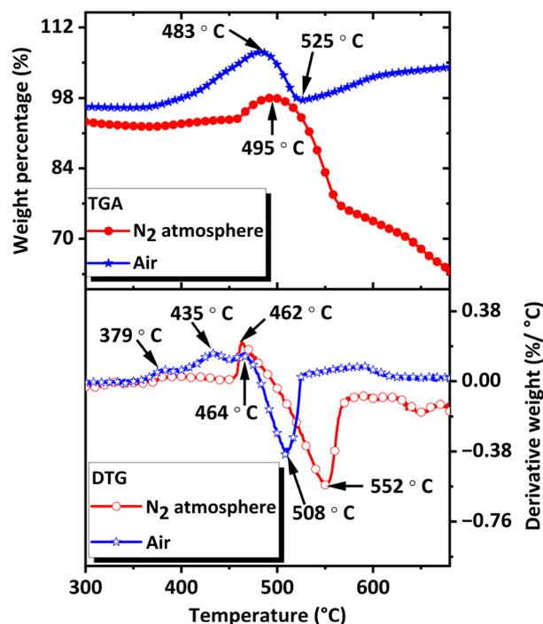
Fig. 8 TGA-DTG curves of CoSb<sub>3</sub> under air and N<sub>2</sub> atmosphere.
