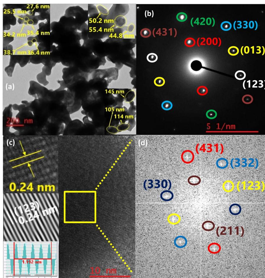
Fig. 5 (a) TEM image of  $\text{CoSb}_3$ , with particles of different morphology in the insets, top left and right-cassini oval-shaped particles, and bottom right-plate-like particles (b) SAED pattern with planes indexed (c) HRTEM image with insets, top left-marked lattice plane, middle-inverse FFT image and the bottom left-simulated calculation result of lattice spacing and (d) FFT image of the marked area.
