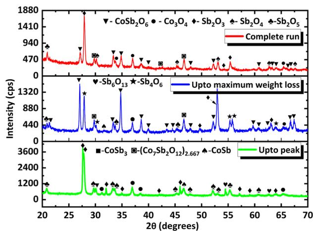
Fig. 13 PXRD data of TGA residues obtained at different stages under a N<sub>2</sub> atmosphere (the stages at which they are collected are provided in the corresponding PXRD pattern).
