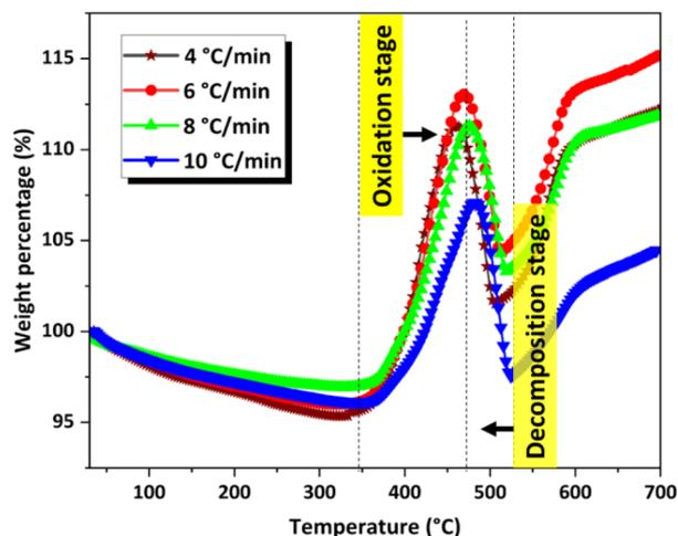
Fig. 9 TGA curves of CoSb<sub>3</sub> in air at different heating rates.
