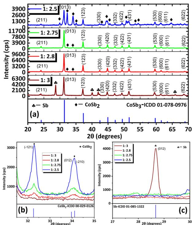
Fig. 1 (a) PXRD pattern of the CoSb<sub>3</sub> samples obtained at different SbCl<sub>3</sub> concentrations (the equivalents of reactants are shown in the corresponding PXRD pattern). (b) 2θ region showing (121), (012) and (210) peaks of CoSb<sub>2</sub> and (c) 2θ region showing (012) peak of Sb.
