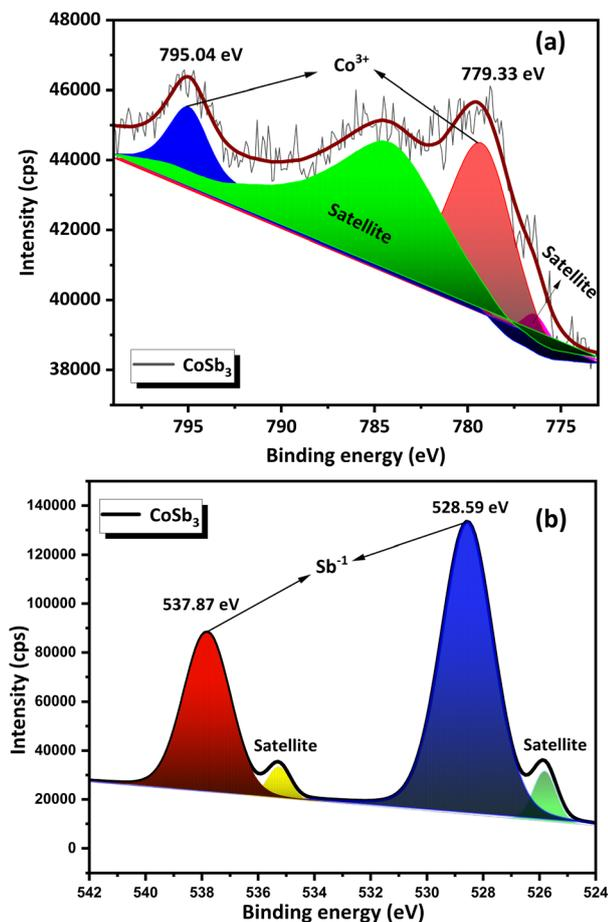
Fig. 7 (a) Narrow scan XPS spectra of Co and (b) Sb in CoSb<sub>3</sub>.
