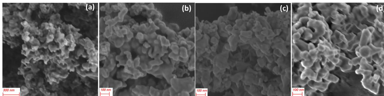
Fig. 4 SEM images of (a)  $\text{CoSb}_3$  obtained at optimized reaction conditions (1:2.8 equivalents of reactants and reaction duration of 72 h), recorded using an SE detector and SEM images showing morphology evolution from cassini oval to plate-like shape over the increment of the reaction duration, (b) 24 h, (c) 48 h and (d) 72 h, recorded using an in lens detector.
