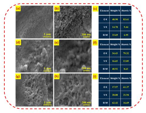
Fig. 7 The scanning electron microscopy images of BiVO<sub>4</sub> thin films (a, b, d, e, g and h) and (c, f and i) EDAX weight and atomic percentages of the substrate temperature-varied BiVO<sub>4</sub> thin films.
