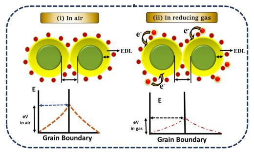
Fig. 12 Chemi-resistive gas sensing mechanism
