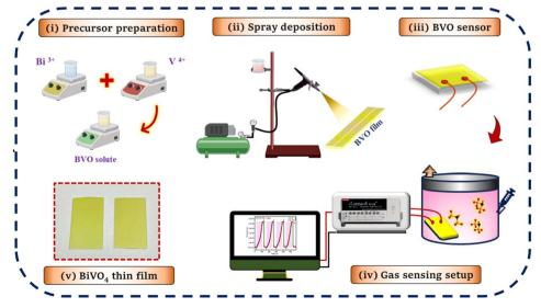
Fig. 1 Schematic diagram of the preparation, deposition and gas sensing measurements of the BiVO<sub>4</sub> thin films.
