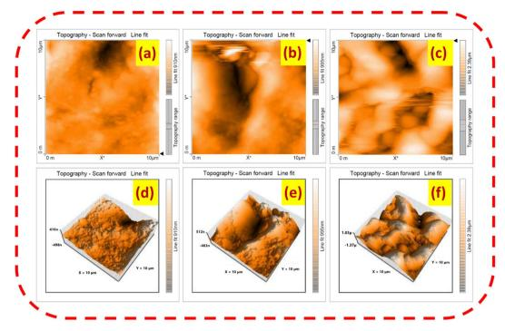
Fig. 5 (a, c and e) and (b, d and f) 2D and 3D topographical images of the substrate temperature-varied BiVO<sub>4</sub> thin films.
