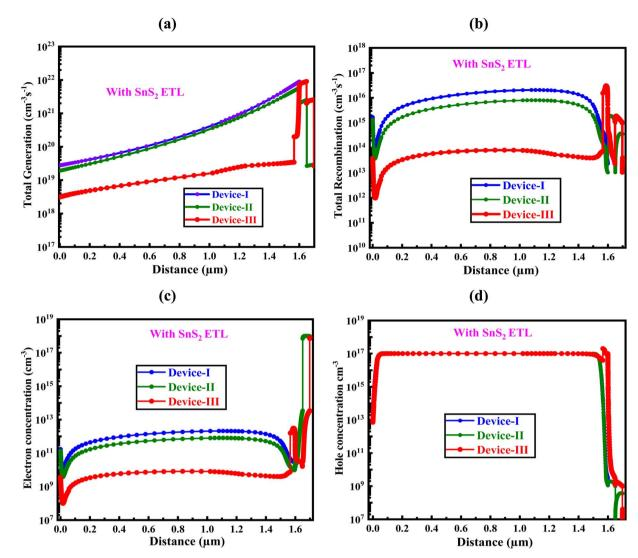
Fig. 14 Influence of absorber layer thickness on (a and b) carrier generation and recombination rates (c and d) electron and hole concentration.
