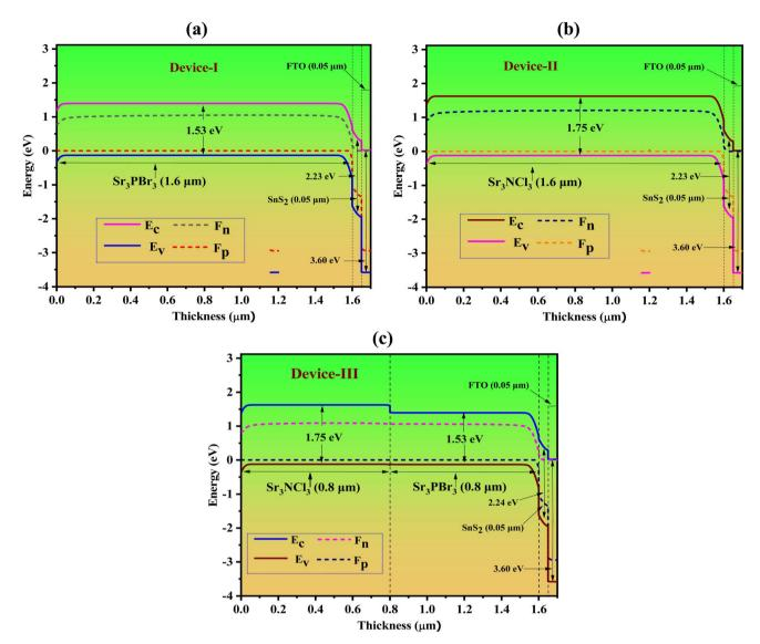
Fig. 3 A band configuration of three varieties of SCs, incorporating various substances that absorb light: (a) Sr<sub>3</sub>PBr<sub>3</sub>, (b) Sr<sub>3</sub>NCl<sub>3</sub>, (c) Sr<sub>3</sub>PBr<sub>3</sub>/Sr<sub>3</sub>NCl<sub>3</sub> bilayer combination.
