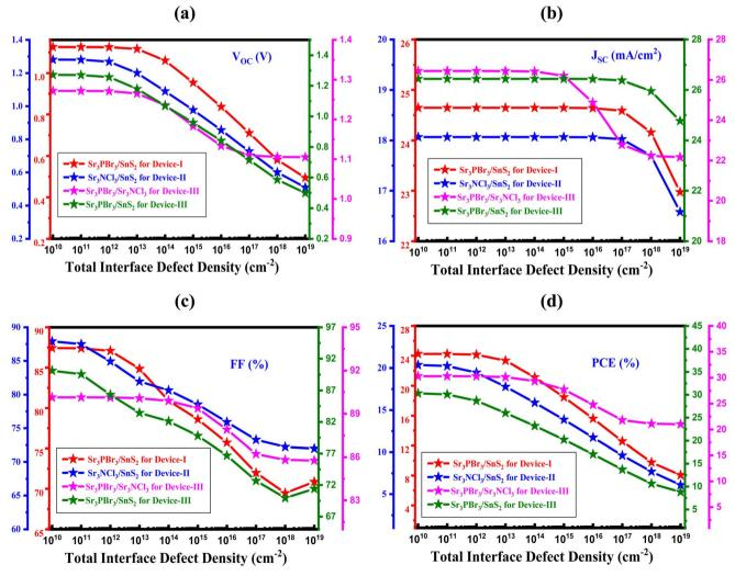
Fig. 8 Effects of interface densities of defect on the performance metrics of the PSC: (a)  $V_{\rm OC}$ , (b)  $J_{\rm SC}$ , (c) FF, and (d) PCE.
