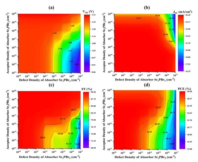
Fig. 6 Effects of the density of bulk defects adjustments vs.  $Sr_3PBr_3$  absorber doping on PV characteristics; (a)  $V_{OC}$  (b)  $J_{SC}$  (c) FF and (d) PCE utilizing  $SnS_2$  as the ETL.
