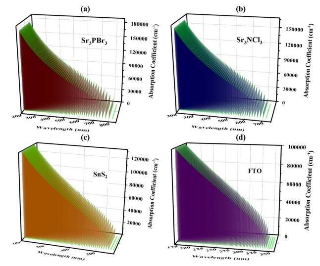
Fig. 12 An analysis of the absorption coefficient is conducted for the ideal SC architecture of FTO/SnS $_2$ /Sr $_3$ PBr $_3$ /Sr $_3$ NCl $_3$ /Ni, specifically for the materials: (a) Sr $_3$ PBr $_3$ , (b) Sr $_3$ NCl $_3$ , (c) SnS $_2$ , and (d) FTO.
