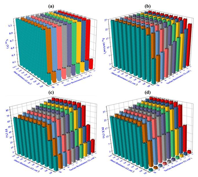
Fig. 10 The contribution of shunt and series resistance to the overall electrical execution of PSCs is demonstrated in terms of (a)  $V_{\rm OC}$ , (b)  $J_{\rm SC}$ , (c) FF, and (d) PCE, specifically for the optimized structure of (FTO/SnS<sub>2</sub>/Sr<sub>3</sub>PBr<sub>3</sub>/Sr<sub>3</sub>NCl<sub>3</sub>/Ni).
