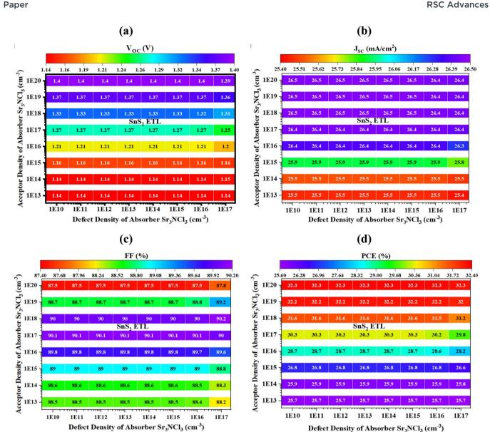
Fig. 7 Effects of the density of bulk defects adjustments vs.  $Sr_3NCl_3$  absorber doping on PV characteristics; (a)  $V_{OC}$  (b)  $J_{SC}$  (c) FF and (d) PCE utilizing SnS<sub>2</sub> as the ETL.
