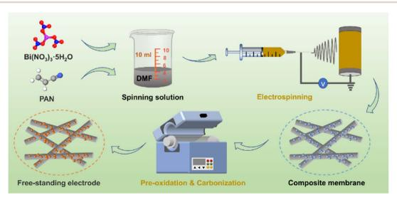
Fig. 1 Schematic diagram of the preparation process for the Bi/CF.
