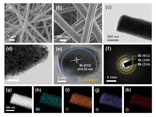
Fig. 2 Microstructure characterization of Bi/CF. (a and b) SEM images. (c) Low and (d) high magnification TEM images. (e) HRTEM and (f) SAED results for Bi/CF. (q-k) The corresponding element mapping of Bi, C, N and O.
