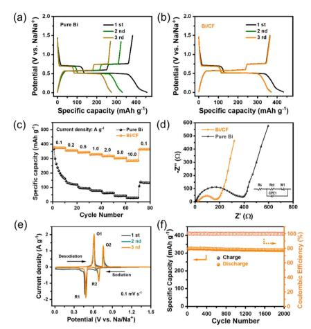
Fig. 4 Electrochemical performance of the electrode. GCD profiles of the (a) Pure Bi and (b) Bi/CF at  $0.1 \text{ A g}^{-1}$ . (c) Rate performance. (d) EIS diagram (the inset shows corresponding equivalent circuit). (e) CV profiles at the scan rate of  $0.1 \text{ mV s}^{-1}$ . (f) Long-term cycles of Bi/CF at current density of  $1.0 \text{ A g}^{-1}$ .
