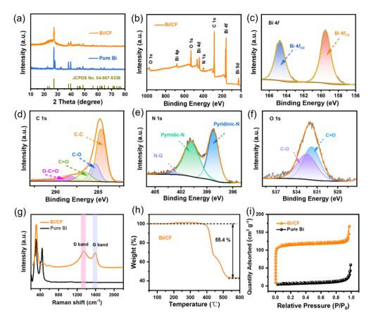
Fig. 3 (a) XRD patterns. (b) XPS spectra. High-resolution of the Bi/CF: (c) Bi 4f, (d) C 1s, (e) N 1s and (f) O 1s. (g) Raman spectra. (h) Thermogravimetric curve. (i)  $N_2$  adsorption/desorption isotherm.
