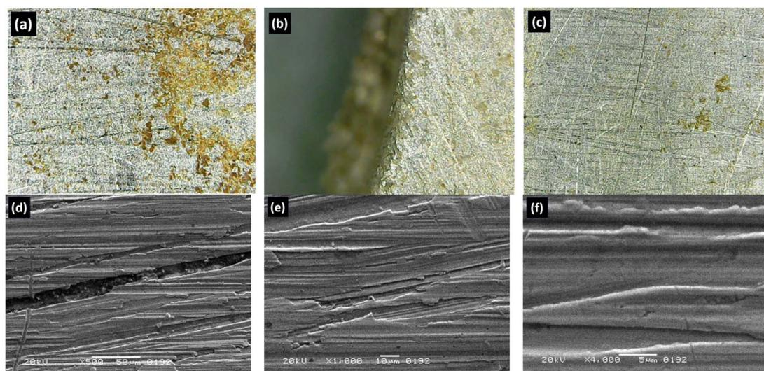
Fig. 7 Digital microscopic and SEM images of different locations of electrodes run on Configuration-1,  $6 \text{ g L}^{-1}$ , after a 10 days run in the HHO generator. Figure (a), (b) and (c) are microscopic images, figure (d), (e) and (f) are SEM images.
