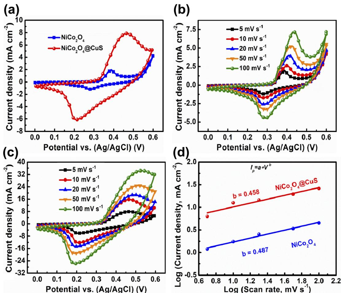
Fig. 5 (a) Comparative CV curves of the as-prepared electrodes at 5 mV s<sup>-1</sup>. CV plots of (b) bare NiCo<sub>2</sub>O<sub>4</sub> and (c) NiCo<sub>2</sub>O<sub>4</sub>@CuS composite electrode. (d) Relationship between the log(*i<sub>p</sub>*) and log(*v*).
