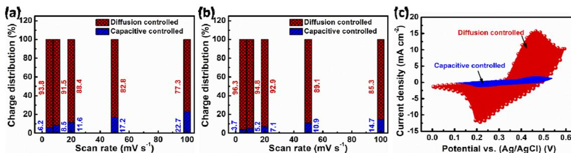
Fig. 6 Diffusion- and capacitive-controlled charge storage contributions in the (a) bare NiCo<sub>2</sub>O<sub>4</sub> and (b) NiCo<sub>2</sub>O<sub>4</sub>@CuS composite electrodes at varying scan rates. (c) Capacitive and diffusion-controlled charge storage contribution breakdown in the NiCo<sub>2</sub>O<sub>4</sub>@CuS composite electrode at 10 mV s<sup>-1</sup>.
