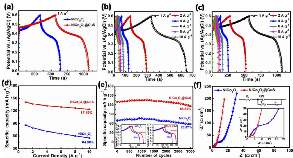
Fig. 7 (a) Comparative GCD plots. GCD curves of (b) bare  $\text{NiCo}_2\text{O}_4$  and (c)  $\text{NiCo}_2\text{O}_4@\text{CuS}$  composite electrode measured at different current densities. (d) Specific capacity values. (e) The cycling life of the electrodes is over 3000 cycles at  $4 \text{ A g}^{-1}$ . The inset shows the initial and final cycles of the cycling test. (f) Nyquist plots of the electrodes, with inset magnifications and an equivalent circuit for fitting the plots.
