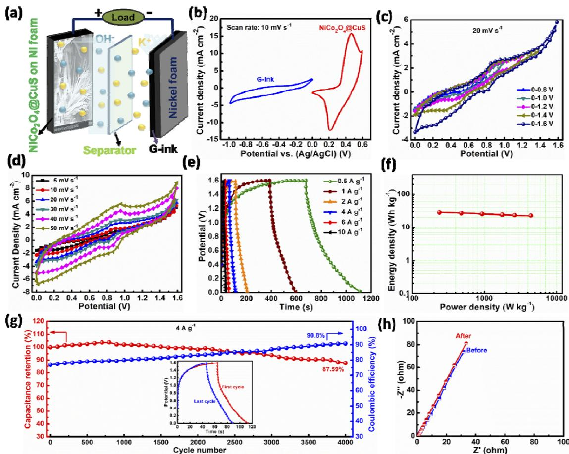
Fig. 8 (a) Schematic representation of the hybrid supercapacitor (HSC) device  $\text{NiCo}_2\text{O}_4\text{@CuS//G-ink}$ . (b) CV plots of both G-ink and  $\text{NiCo}_2\text{O}_4\text{@CuS}$  electrodes at  $10 \text{ mV s}^{-1}$ . (c) CV plots of the HSC device under different potential regions at  $20 \text{ mV s}^{-1}$ . (d) CV, (e) GCD, (f) Ragone plot, and (g) cycling stability of the HSC device. (h) EIS Nyquist plots of the HSC device before and after the cycling stability test.
