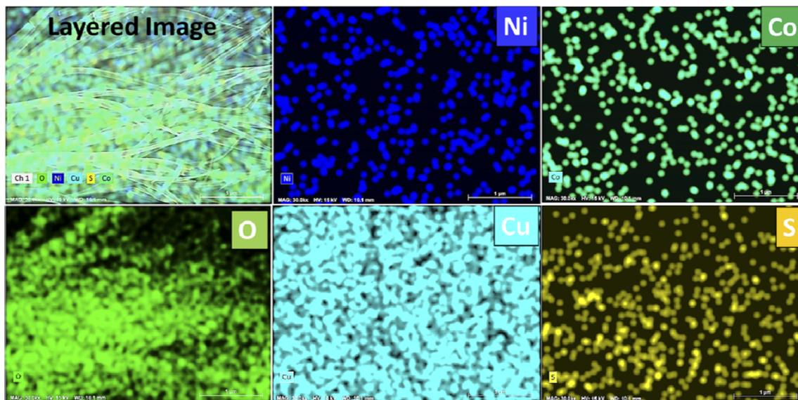
Fig. 2 EDS mapping images of NiCo<sub>2</sub>O<sub>4</sub>@CuS composite electrode.
