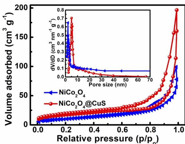
Fig. 4 N<sub>2</sub> adsorption–desorption isotherm of the bare NiCo<sub>2</sub>O<sub>4</sub> and NiCo<sub>2</sub>O<sub>4</sub>@CuS composite electrodes. The inset shows the BJH pore size distribution.
