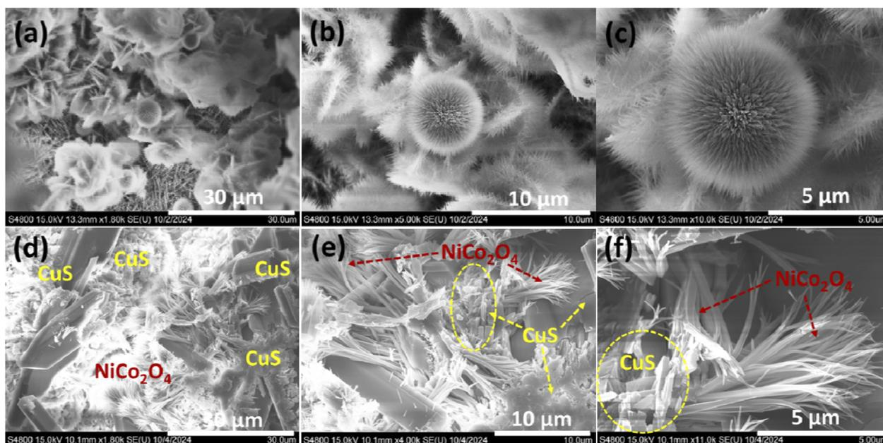
Fig. 1 FE-SEM images of (a–c) NiCo<sub>2</sub>O<sub>4</sub> and (d–f) NiCo<sub>2</sub>O<sub>4</sub>@CuS composite at various magnifications.
