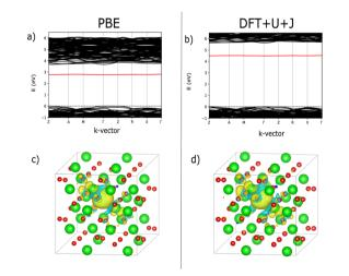
Fig. 1 Comparison of defect bandstructure and electron localisation for the charge neutral 3-fold O vacancy in  $ZrO_2$ . (a) Defect bandstructure for the PBE structure. (b) Defect bandstructure for the DFT+U+J structure. (c) Electron localization for the PBE structure. (d) Electron localization for the DFT+U+J structure. (c and d) Were calculated from the difference in charge density values between +0 and +2 calculations on the same +0 geometry.
