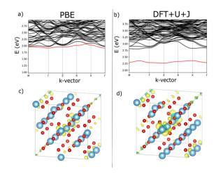
Fig. 7 Visualisation of the electronic and localisation properties of the charge neutral O vacancy for rutile TiO2, using PBE or DFT+U+J. (a and b) Shows, for PBE and DFT+U+J respectively, the bandstructure of the defective cell near the CBM with the lowest defect band in the vicinity of the CBM highlighted in red. Figures (c and d) show, for PBE and DFT+U+J respectively, the difference in charge density for a relaxed defective cell between the charge neutral and charge +2 cases.
