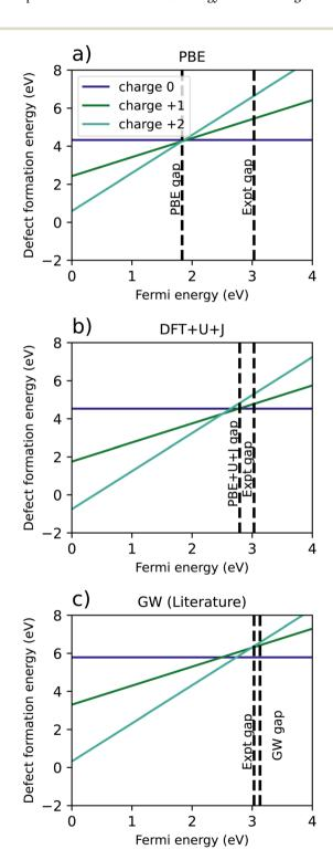
Fig. 8 Comparison of defect formation energies for TiO<sub>2</sub> calculated using (a) PBE functional, (b) DFT+U+J functional, (c) a recreation of G0W0 results from Malashevich et al. 47
