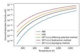
Fig. 6 The predicted concentrations under different temperatures of O vacancy defects in HfO2 under O rich conditions. The HSE results were derived from Lyons et al.40 The "naïve" method has been omitted for giving unphysical results. The dominant defect for all methods was the +2 charged 3-fold coordinated O vacancy.
