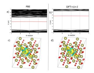
Fig. 4 Comparison of defect bandstructure and electron localisation for the charge neutral 3-fold O vacancy in  $HfO_2$ . (a) Defect bandstructure for the PBE structure. (b) Defect bandstructure for the DFT+U+J structure. (c) Electron localisation for the PBE structure. (d) Electron localisation for the DFT+U+J structure. Figures (c and d) were calculated from the difference in charge values between +0 and +2 calculations on the same geometry.
