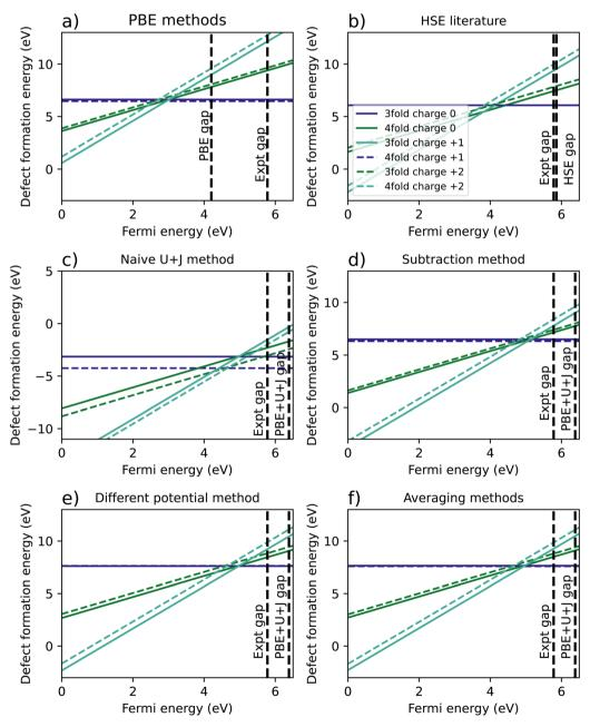
Fig. 5 Calculated defect formation energies for HfO<sub>2</sub> under 6 different methodologies. (a) Shows the regular PBE method, (b) is a from Lyons et al.<sup>40</sup> (c) refers to a naïve DFT+U+J calculation without corrections for differing U+J values on O atoms, and (d-f) refer to three different methods of correcting for these U+J values.
