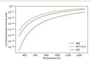
Fig. 9 Predicted defect concentrations under different temperatures for TiO2 under O rich conditions. Only the dominant +2 charged O vacancy defect is shown. GW results are derived from the defect formation energies of Malashevich et al.47
