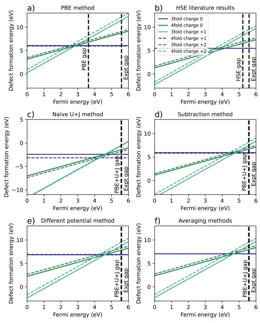
Fig. 2 A comparison of calculated defect formation energies for ZrO<sub>2</sub> under different methodologies. (a) Shows the regular PBE approximation, (b) is from Lyons et al. (c) refers to a naïve DFT+U+J calculation without corrections for differing U+J values on O atoms, and (d-f) refer to three different methods of correcting for these U+J values.
