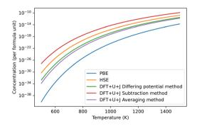
Fig. 3 Predicted concentrations in  $ZrO_2$  of the dominant O defect for different temperatures, under all different techniques, under O rich conditions. The HSE results were derived from Lyons *et al.*<sup>40</sup> The "naïve" method was omitted as it produced unphysical predictions. In all cases shown in the figure this dominant defect was the +2 charged 3-fold coordinated O vacancy.
