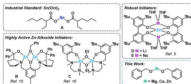
Fig. 1 Examples of the industrial standard Sn(Oct)<sub>2</sub>, highly active and/or robust Zn-alkoxide initiators, and the simple salts explored for LA ROP in this work.<sup>4,5,14,15</sup>
