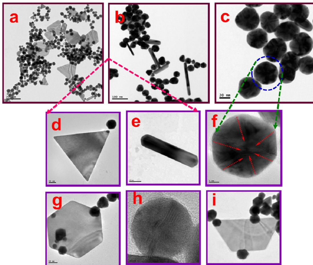
Fig. 4 HR-TEM images for (a–c) controlled shapes of anisotropic oligo AMTa-AuNS synthesized by 500  $\mu\text{L}$  AMTa addition at 80  $^{\circ}\text{C}$  reaction temperature and (d–i) HR-TEM images of magnified view of (d) triangle, (e) rod, (f) pyramid, (g) hexagonal (h) spherical and (i) boat shaped anisotropic oligo AMTa-AuNS.
