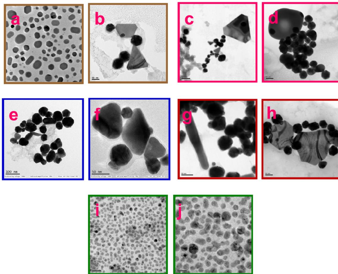
Fig. 5 HR-TEM images uncontrolled growth of anisotropic oligo AMTa-AuNS synthesized by (a and b) 1 mL AMTa at 80 °C, (c and d) 2 mL AMTa at 80 °C, (e and f) 500  $\mu$ L AMTa at 60 °C, (g and h) 500  $\mu$ L AMTa at 100 °C and (i and j) pure AuNPs.
