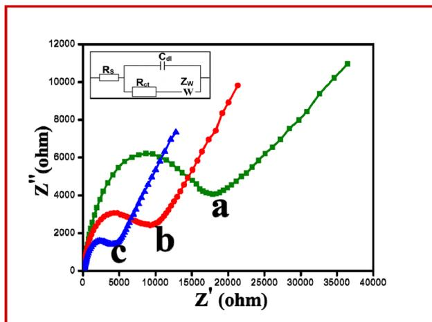
Fig. 7 A Nyquist plot for (a) unmodified GC, (b) GC/oligo AMTa, and (c) GC/oligo AMTa-AuNS electrodes in 1 mM  $K_3[Fe(CN)_6]/K_4[Fe(CN)_6]$  containing 0.2 M PB solution (pH 7.2) at scanning frequencies from 0.01 to 100 000 Hz.
