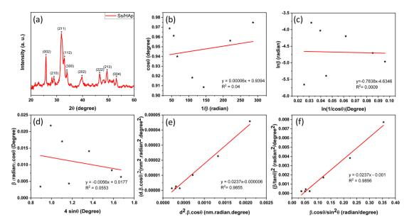
Fig. 2 (a) XRD pattern of Ss/nHAp, linear fit plot of (a) LSLM, (b) MSM, (d) WHM, (e) SSPM, and (f) HWM for calculating crystallite size of synthesized Ss/nHAp.
