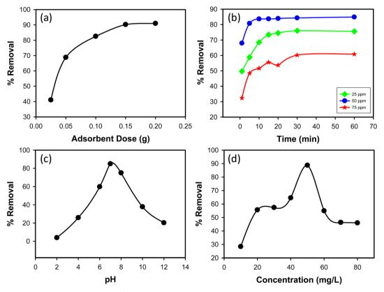
Fig. 6 (a) Effect of adsorbent dose ( $C_0 = 50 \text{ mg L}^{-1}$ , time = 30 min, pH = 7, shaking speed = 200 rpm); (b) effect of contact time ( $C_0 = 25, 50 \text{ }60, 50$
