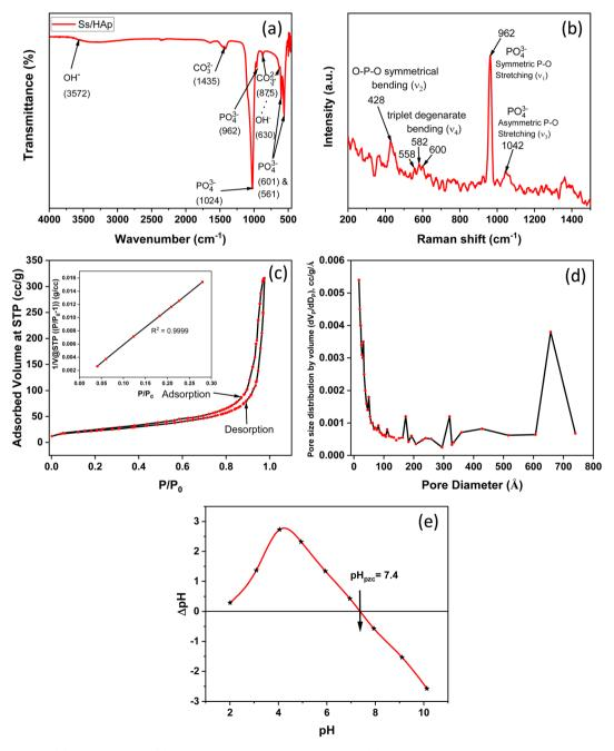
Fig. 4 (a) FTIR spectra, (b) Raman spectra, (c)  $N_2$  adsorption—desorption isotherm, (d) BJH adsorption pore size distribution curve, and (e) point of zero charge (pH<sub>pzc</sub>) determination of Ss/nHAp.
