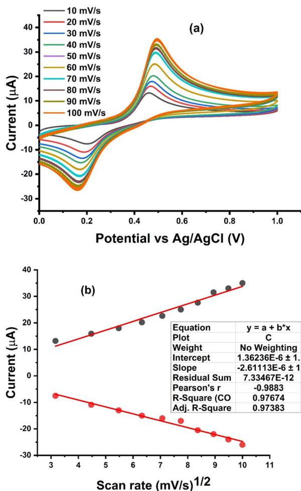
Fig. 6 (a) Redox peak current response of Ni-Al-LDH/GCE at various scan rates in a 0.1  $\mu\text{M}$  PCT solution utilizing BRB at pH 3. (b) Graph depicting the relationship between the square root of the scan rate and the redox peak current.
