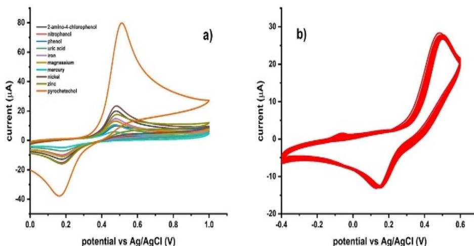
Fig. 8 (a) Effect of different interferences on the sensor response at a 0.1  $\mu\text{M}$  PCT concentration. (b) Thirty consecutive runs of the Ni–Al-LDH/GCE sensor in 0.1  $\mu\text{M}$  PCT to test its stability and consistency.
