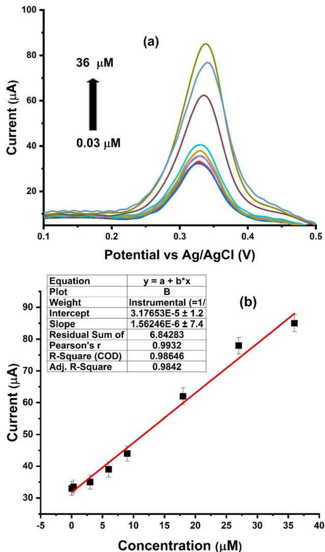
Fig. 7 (a) Peak current response related to PCT concentration, ranging from 0.03–36  $\mu\text{M}$ . (b) Peak current response is a straight line with an  $R^2$  value of 0.986 at an 80  $\text{mV s}^{-1}$  pulse amplitude.
