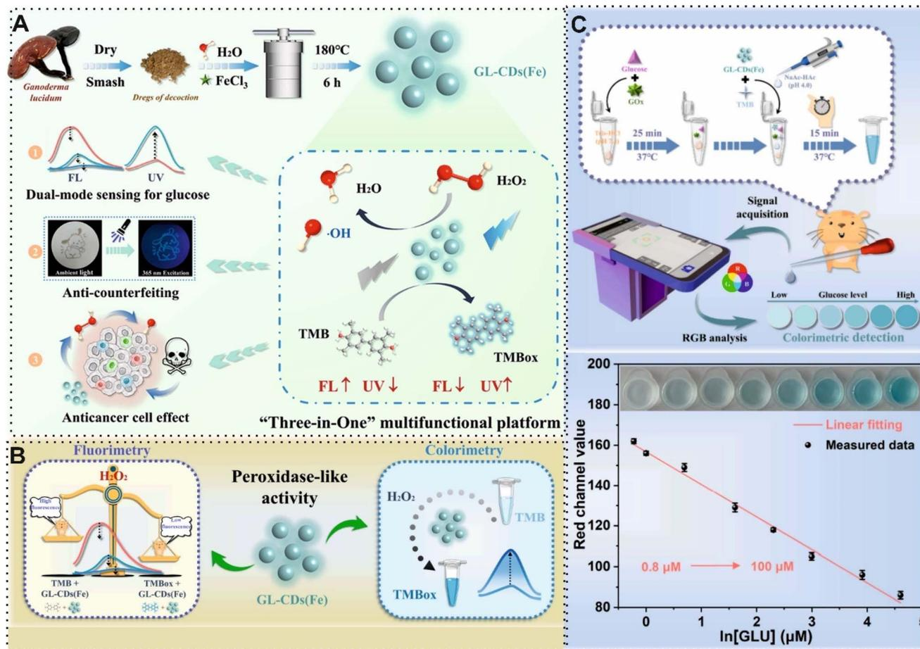
Fig. 4 (A) Representation of using CDs, which derived from *Ganoderma lucidum* waste, for introducing "three-in-one" platform and (B and C) dual-mode sensing platform and integration of smartphone for detection of glucose. Reproduced with permission from ref. 80. Copyright Elsevier Science, 2024.
