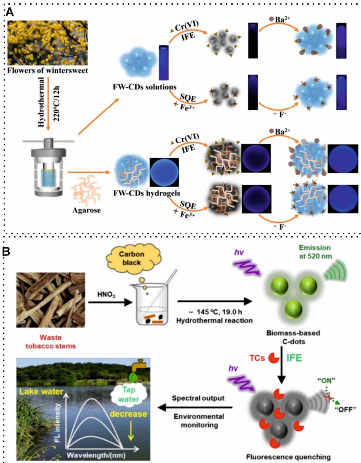
Fig. 8 (A) Schematic of fluorescence sensor based on using flowers of wintersweet for synthesizing CDs for visual quantification of Cr(VI) and Fe<sup>3+</sup>.<sup>92</sup> (B) Illustration of CDs derived from tobacco stems waste for quantification of tetracycline antibiotic residues in water samples.<sup>93</sup>
