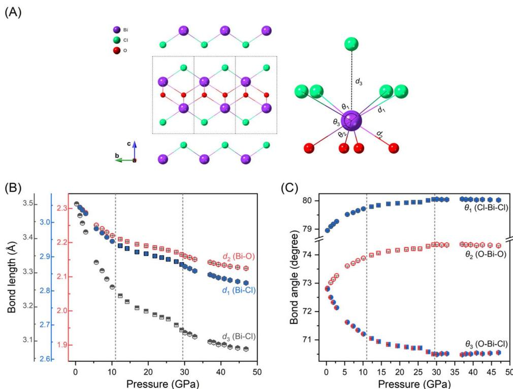
Fig. 5 (A) Schematic illustrations of bond angles and bond lengths of BiOCl. (B) Evolution of Bi–O and Bi–Cl bond lengths under compression. The relative values of the right and left axes are consistent. (C) Bond angles evolution of Cl–Bi–Cl, O–Bi–O and O–Bi–Cl, respectively. With pressure increasing, the in-plane bond angles of Cl–Bi–Cl and O–Bi–O increases, while the out-of-plane bond angle decreases.
