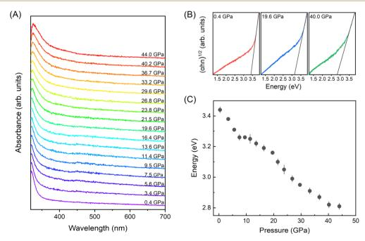
Fig. 2 (A) High-pressure UV-vis absorption spectra of BiOCl nanosheets. (B) Plot of  $(\alpha h v)^{1/2}$  versus photon energy at the selected pressures of 1.3 GPa (left), 19.3 GPa (middle) and 39.7 GPa (right). The dash lines are shown to estimate the optical bandgap. (C) Pressure dependent bandgap. The error bars are estimated from the liner fitting error.
