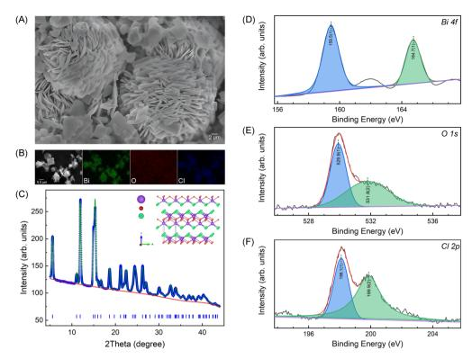
Fig. 1 SEM image (A) and EDS mappings (B) of the synthesized BiOCl nanosheets. (C) 1D XRD pattern along with the Rietveld refinement result using the GSAS-II software package<sup>24</sup> and the inserted shows the layered crystal structure of BiOCl. (D)-(F) are XPS spectra of Bi 4f, O 1s and Cl 2p, respectively.
