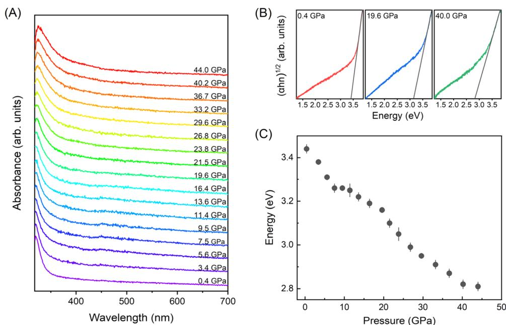
Fig. 2 (A) High-pressure UV-vis absorption spectra of BiOCl nanosheets. (B) Plot of  $(\alpha h\nu)^{1/2}$  versus photon energy at the selected pressures of 1.3 GPa (left), 19.3 GPa (middle) and 39.7 GPa (right). The dash lines are shown to estimate the optical bandgap. (C) Pressure dependent bandgap. The error bars are estimated from the linear fitting error.
