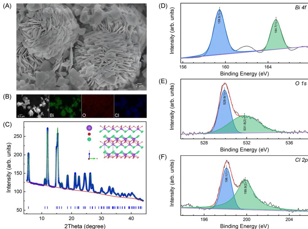
Fig. 1 SEM image (A) and EDS mappings (B) of the synthesized BiOCl nanosheets. (C) 1D XRD pattern along with the Rietveld refinement result using the *GSAS-II* software package<sup>24</sup> and the inserted shows the layered crystal structure of BiOCl. (D)–(F) are XPS spectra of Bi 4f, O 1s and Cl 2p, respectively.
